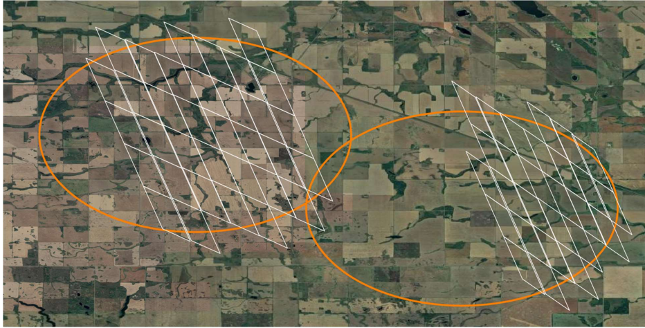
590 591 Figure 6. Overlapping GOSAT and OCO-2 soundings near Quill Lakes, Saskatchewan, Canada. Orange 592 circles are GOSAT sounding footprints (~10 km) and the white rhomboids are OCO-2 sounding 593 footprints (~1.3 km ×by 2.25 km) acquired on the same day as the GOSAT soundings in which they fall. 594 The GOSAT and OCO-2 soundings on the left were acquired in February 2019, and the soundings on the 595 right were acquired in July 2017. The base map is a Google Satellite image. 596
