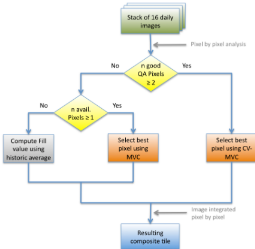
Fig. 2. MODIS compositing algorithm data flow (from Didan et al. 2015).
