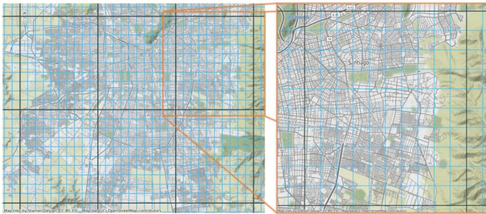
Figure 3 Map of Santiago at different scales: in blue the utilized 0.01^\circ \times 0.01^\circ grid (approximately 1x1 km), and in black the 0.1^\circ \times 0.1^\circ EDGAR V5.0 grid for comparison. © OpenStreetMap contributors 2021. Distributed under the Open Data Commons Open Database License (ODbL) v1.0
