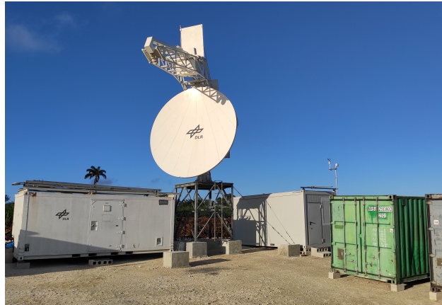
Figure 2. C-band radar Poldirad on Barbados (photo by F. Ewald).
