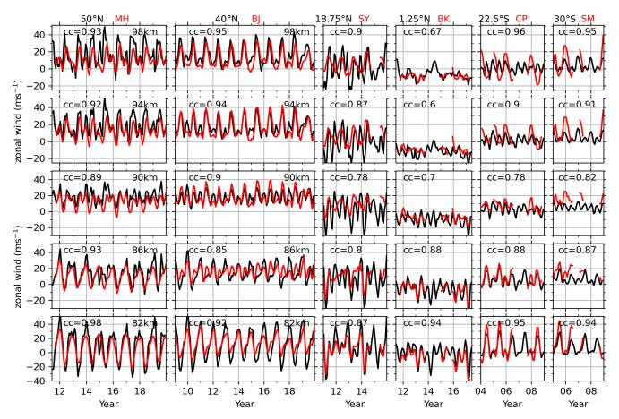
**Figure 8**. Monthly mean zonal wind from meteor radars (red lines, positive for eastward) at stations (from left to right) of MH (53.5°N), BJ (40.3°N), SY (18.3°N), BK (1.2°S), CP (22.7°S) and SM (29.7°S) and the BU (black) at the similar latitude (labeled on the top of each column) at five heights. The correlation coefficient (cc) between BU and MetU is labeled on each panel. Same y-axis is used in each row. The x-ticks mark the beginning of each year.
