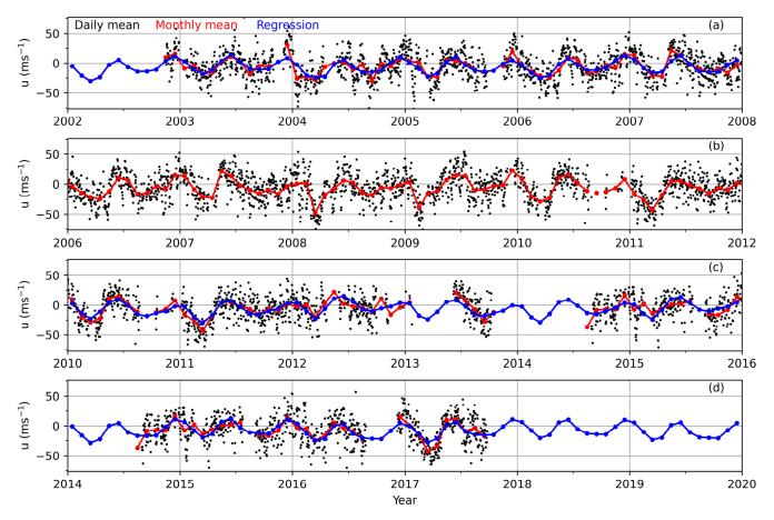
**Figure 1.** The daily mean (black dots) and monthly mean (red line with dots) zonal winds (positive for eastward) at 86 km measured by the JPNKT meteor radar and their regression results (blue line with dots) from 2002 to 2019. The x-ticks mark the beginning of each year.
