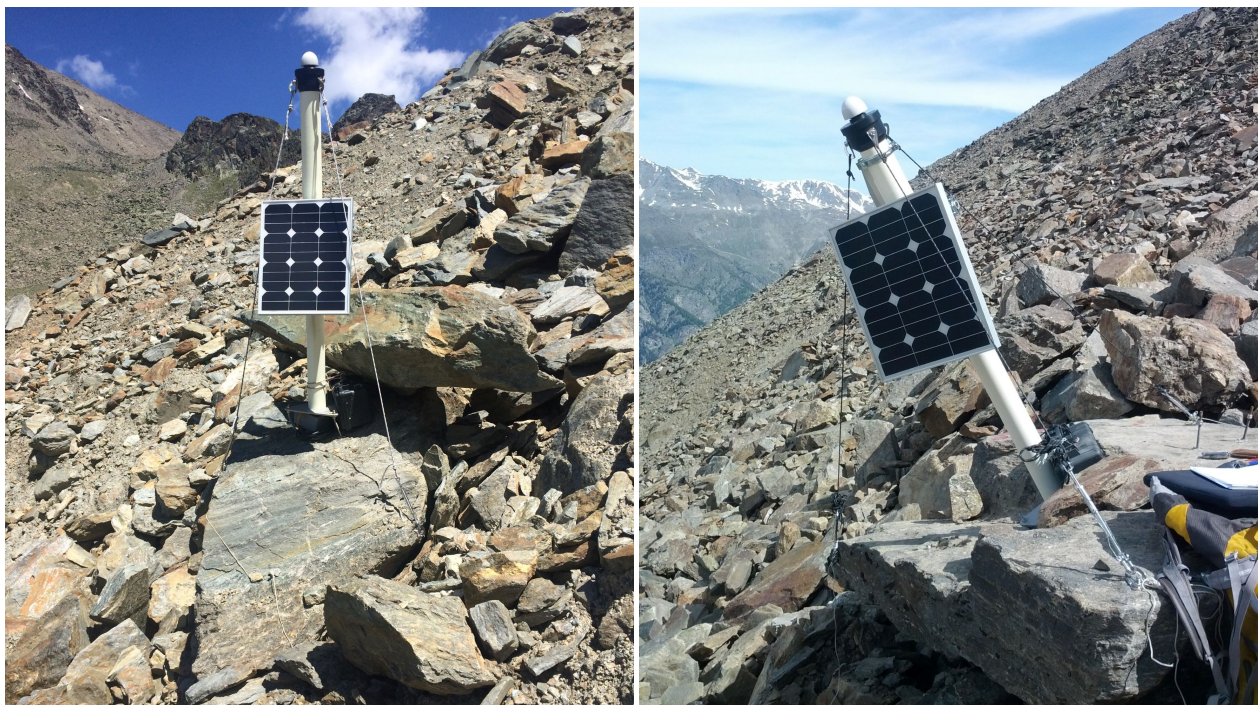
Figure 11. In very active movement zones finding a single block to fix the measurement instrument can be challenging both w.r.t. longevity and w.r.t. the representativeness of the block selected for the movement of the larger landform in question. The two locations shown are very active zones in steep, frontal parts of two rock glaciers above Herbruggen (Switzerland): Dirruh horn rock glacier (left) and Breithorn/Bielzug rock glacier (right). © PermaSense Project
