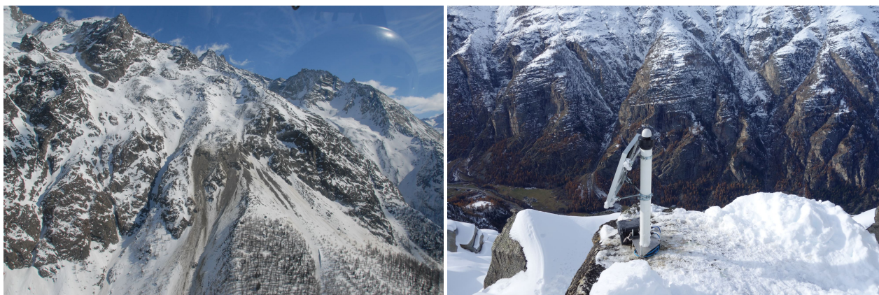
Figure 2. The Grabengufer rock glacier is issuing significant material during a surge period in winter 2009 is fed from a landslide in the snowy depression above where 5x GNSS locations are present, Randa (Switzerland) (left). A GNSS sensor monitoring the terrain movement in the area of Längschnee 2588 m a.s.l. above the village of Herbruggen (Switzerland) (right). © PermaSense Project
