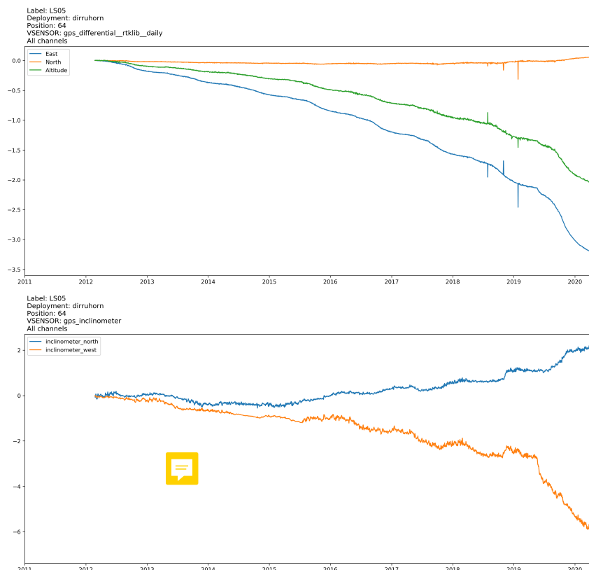
Figure 7. Daily coordinate series in east, north, altitude (top) as well as two-axis daily inclination values (bottom) for an accelerating landslide at Längschnee, Herbriggen (Switzerland) at 2611 m a.s.l. capture the kinematics in five degrees of freedom.
