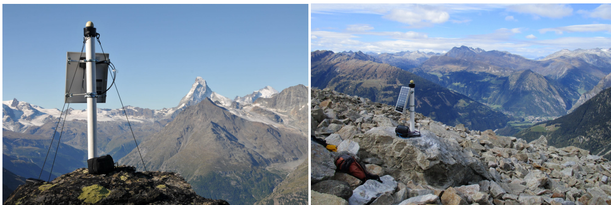
Figure 1. Two GNSS sensing devices mounted atop large boulders found on the landforms being monitored. Breithorn Landslide 2982 m a.s.l., Herbruggen (Switzerland) (left); Largario rock glacier 2355 m a.s.l., Blenio (Switzerland) (right). © PermaSense Project
