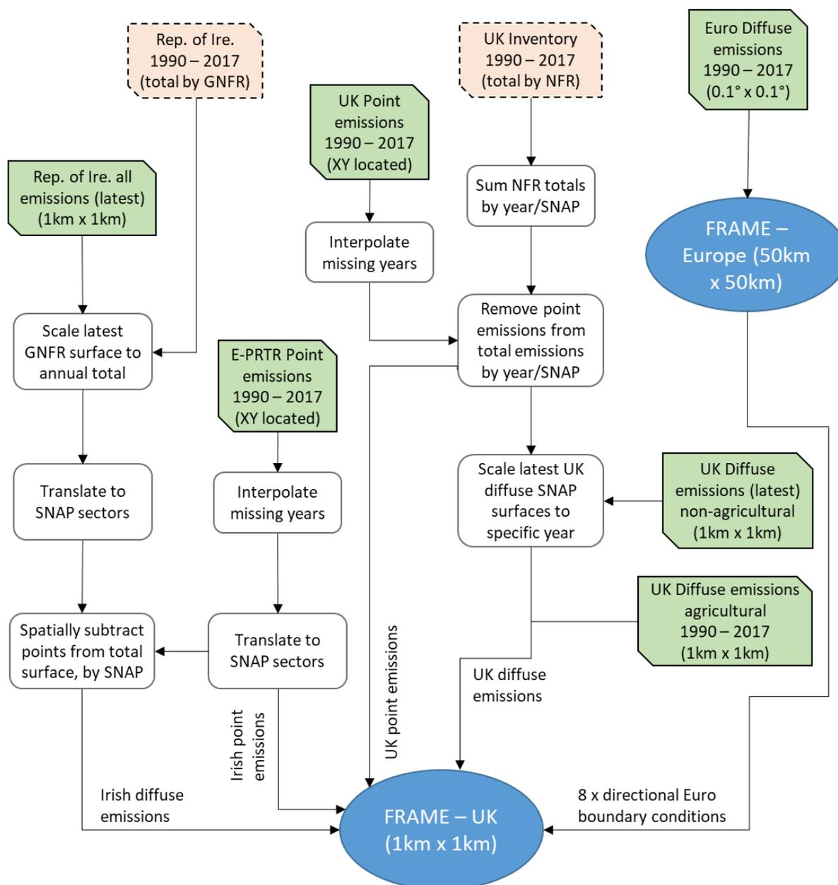
150 Figure 2. Visualised methodology of steps to create inputs for the Fine Resolution Multi-pollutant Exchange (FRAME) atmospheric chemistry transport model; rectangle with corners missing (solid border) = spatial data, rectangle with corners missing (dashed border) = tabulated data, rectangle with rounded corners = process, oval = model.
