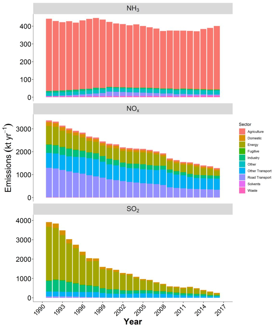
245 Figure 4. Emissions (in kt) of ammonia (NH<sub>3</sub>), nitrogen oxides (NO<sub>x</sub>) and sulphur dioxide (SO<sub>2</sub>) in the model domain, covering the UK and Ireland, from 1990 to 2017, split into the main broad reporting sectors.
