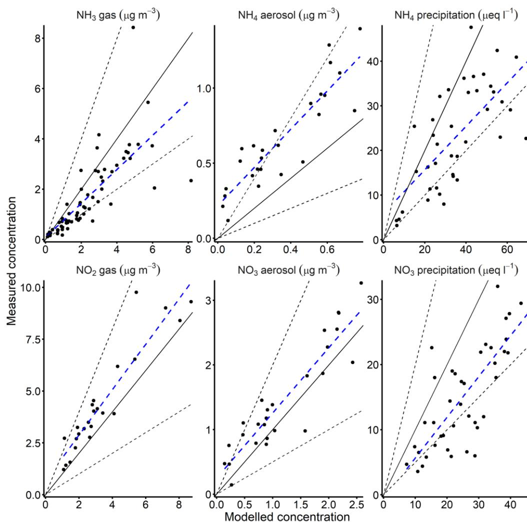
Figure 5: Evaluation of modelled (x-axis) and measured (y-axis) concentrations of six nitrogen compounds in the UK for 2017 (see Table 3 for definitions). The solid black line represents a 1:1 relationship, and the dotted lines represent a factor of two (FAC2) relationship, the blue dashed lines are linear regressions.
