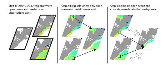
Figure 3. Schematic illustration of the merging steps. Step 1 shows an illustrative example of one  $30^{\circ}x30^{\circ}$  box that includes both coastal and open ocean SOCAT observations. in Step 2 empty grid cells within the 30°x30° box are filled with coastal ocean as well as open ocean datapoints and in Step 3 open ocean and coastal ocean datapoints are combined where both exist.
