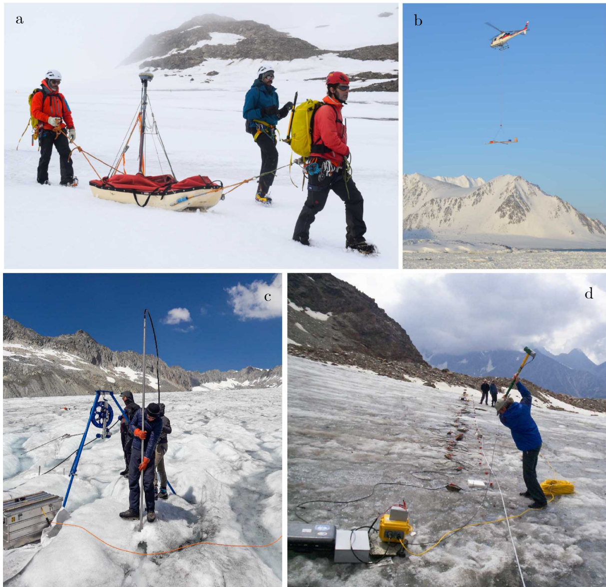
Figure 1. Field photographs illustrating different methods for measuring glacier thickness. (a) Ground-penetrating radar measurements on Johnsons Glacier, Antarctica, in January 2020. The white sledge contains a radar transmitter, receiver, shielded antennas, control unit, and recording system. A Global Navigation Satellite System receiver antenna is mounted to the sledge. Credit: Francisco Navarro. (b) Aerial ground-penetrating radar measurements over Hansbreen, Svalbard, in spring 2011 (Navarro et al., 2014). The radar transmitter, receiver, and antennas are mounted to a wooden frame hung from the helicopter. Credit: Antoine Kies. (c) Hot water drilling on Rhonegletscher, Switzerland, in August 2018 by ETH Zurich’s Glacier Seismology Group. Although used mostly for characterizing bed conditions, the drillings measure ice thickness as a side product. Credit: Johannes Landmann. (d) Seismic reflection measurements on Grubengletscher, Switzerland, using a sledgehammer as a seismic energy source. The black seismic line connects geophones to the recording system. Credit: Bernd Kulesa.
