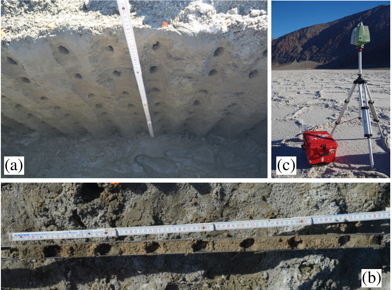
Figure 4. Field methods. (a) Representative trench and sampling positions (holes) at a site at Owens Lake. (b) Dutch gouge auger and sampling positions (holes) at a site at Owens Lake (crust-soil interface is positioned at 0 cm). (c) Terrestrial Laser Scanner (TLS) setup at Badwater Basin.
