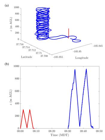
**Figure 2.** Flight profiles for first flights conducted by BCT5D (blue) and SOLOW (red) at Zulu on July 15, 2018 illustrating typical flight profiles for fixed-wing and rotorcraft UAS at sampling sites on July 15, 16 and 18. Flight trajectories in spatial domain shown in (a), with (b) showing the altitude above ground level of each aircraft as a function of time.
