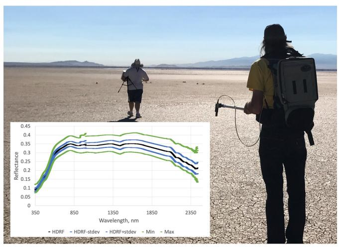
Figure 9 Surface characterization on October 25<sup>th</sup>, 2017 at Rosamond Dry Lake in California using a Spectralon reflectance standard and ASD FieldSpecPro. (Inset) Mean and standard deviation of surface reflectance (black, blue lines) with maxima and minima spectra (green).
