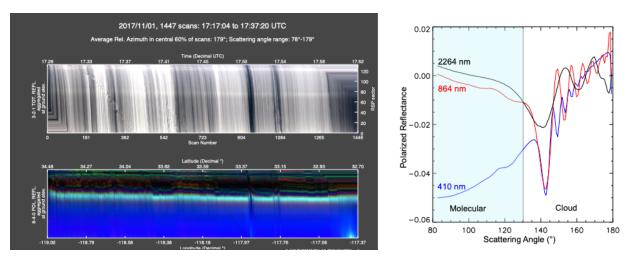
Figure 6 RSP quick look image (left) from November 1st, 2017. The vertical dimension represents view angle, and the horizontal dimension scan number (time elapsed. At right is a single level 1C scan corresponding to scan 1235 at left. It shows the signature of cloud bows at large scattering angles (135-180°) and molecular (Rayleigh) scattering for 410 nm at scattering angles smaller than 130°. Retrieved droplet size parameters are effective radius of 11.5 µm and effective variance of 0.008.
