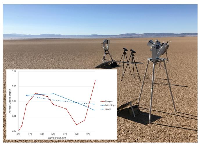
Figure 8 GroundMSPI, two Microtops sunphotometers, and a University of Arizona Reagan sunphotometer deployed on October 25<sup>th</sup>, 2017 at Rosamond Dry Lake in California. (Inset) AOD as measured by the Microtops and Reagan sunphotometers.
