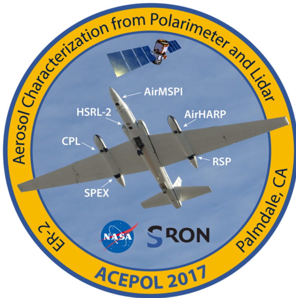
Figure 3 The ACEPOL field campaign emblem, which also shows the positions of instruments onboard the ER-2 aircraft.
