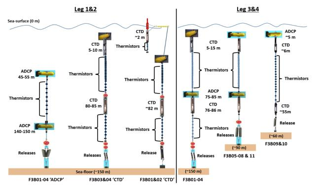
Figure 2: DFO taut line moorings, leg1&2 (left), leg 3&4 (right). In leg 2, F3B01&2 'CTD' lines were converted to F3B03&04's design due to failures of the sea-surface part. A 110 m rope, without thermistors, was added under the bottom CTD of F3B08 to be deployed
