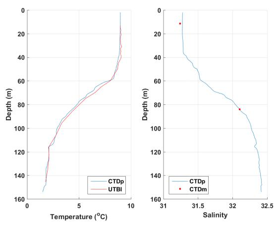
Figure 6: in-situ CTD profile (CTDp) comparison with moored thermistors (UTBI) and CTD (CTDm) on November DD, 2016 at F3B01
