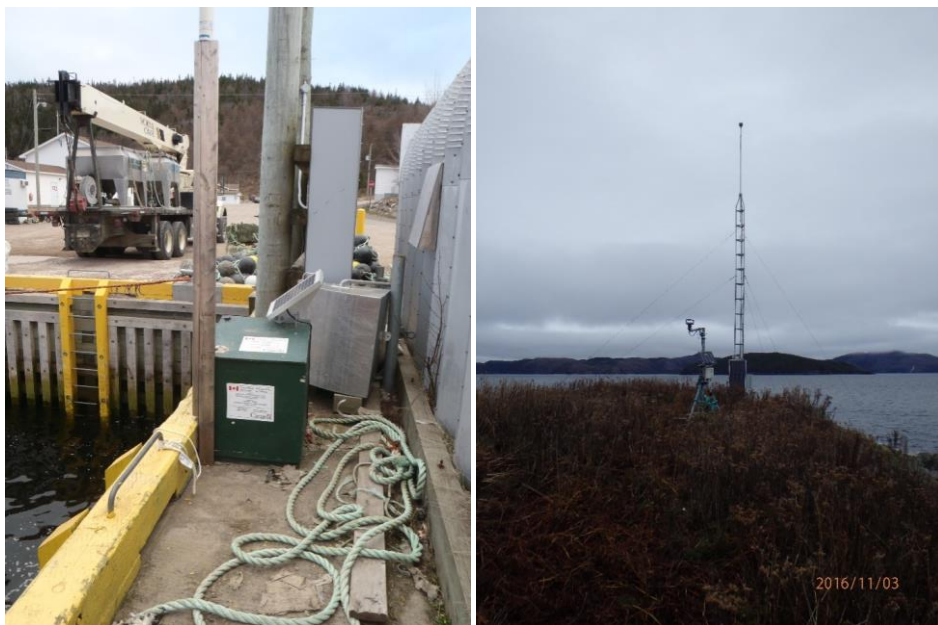
Figure A-1: Pool's Cove (POOLC) tide gauge (left) and Dog Island (DOGIS) weather stations (right)
