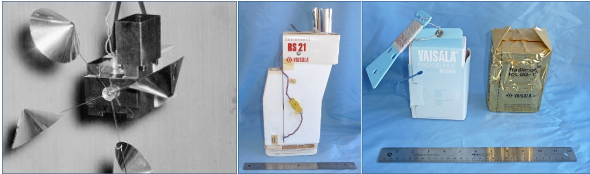
155 Figure 1: Three types of Vaisälä radiosondes. Left: The Vaisälä RS-11 was introduced in 1937 and won a gold medal in the world fair at Paris (vaisala.com). Middle: Vaisälä RS-21 from 1971 (radiosondemuseum.org). Right: Vaisälä RS-80-N from 1981 with its original packaging (radiosondemuseum.org). All three radiosondes have been used in the intercomparison campaigns in our collection. They correspond to comp002fin (left), comp009van (middle) comp009v80 (right). Note, that the introduction dates may vary because of slight modification of the instruments.
