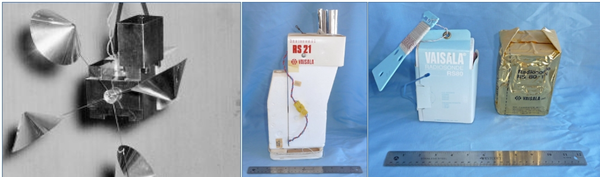
Figure 1: Left: Three types of Vaisälä radiosondes. Left: : The Vaisälä RS-11 was introduced in 1937 and won a gold medal in the world fair at Paris (vaisala.com). Middle: Vaisälä RS-21 from 1971 (radiosondemuseum.org). Right: Vaisälä RS-80-N from 1981 with its original packaging (radiosondemuseum.org). All three radiosondes have been used in the intercomparison campaigns in our collection. They correspond to comp002fin (left), comp009van (middle) comp009v80 (right). Note, that the introduction dates may vary because of slight modification of the instruments.
