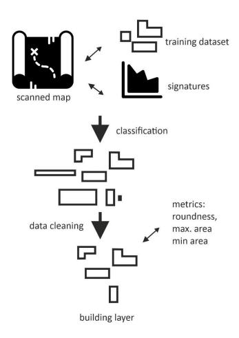
365 Figure 3: Semiautomatic procedure for acquiring residential building structures (originally marked with red) from historical maps.
