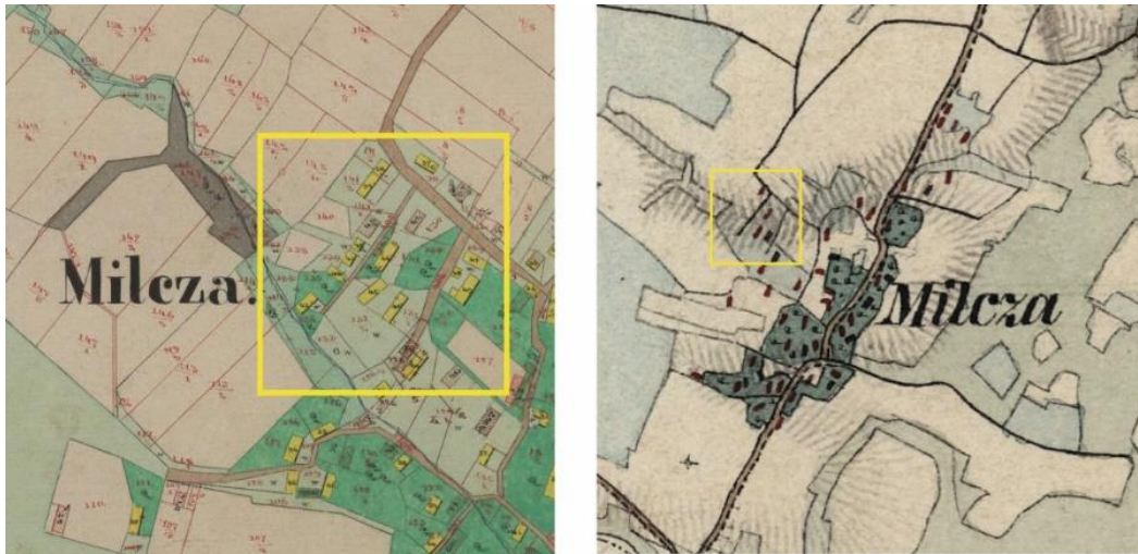
560 Figure 87: Comparison of a cadastral map (1851) and Second Military Survey map (1861/62) that indicates a very high level of map generalization; (source: National Archive in Przemyśl, Austrian States Archives War Archive Vienna ).
