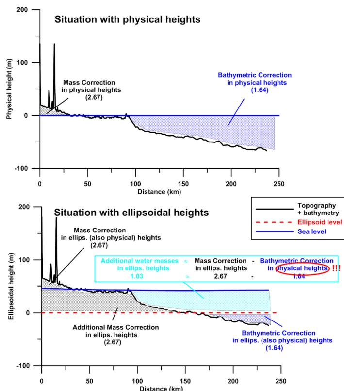
695 **Figure 7: Schematic comparison of ellipsoidal vs. physical concept of CBA. Note that the effect of additional water masses is calculated in a two-step process.**
