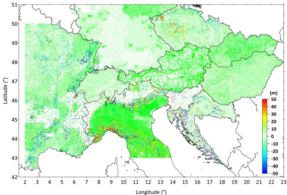
565 **Figure 3:** Height differences (in meters) for gravity stations in the "inner zone" of the TOPOSK software (refer to Sect. 4.1) between the used DEMs and the heights of these stations.
