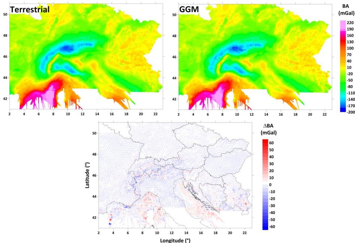
1100 **Figure 20: Comparison of Bouguer anomaly maps (correction density  $2670 \text{ kg m}^{-3}$ ) derived from terrestrial data (upper left) and GGM model EIGEN-6C4 (upper right). The bottom map shows the difference between the two.**
