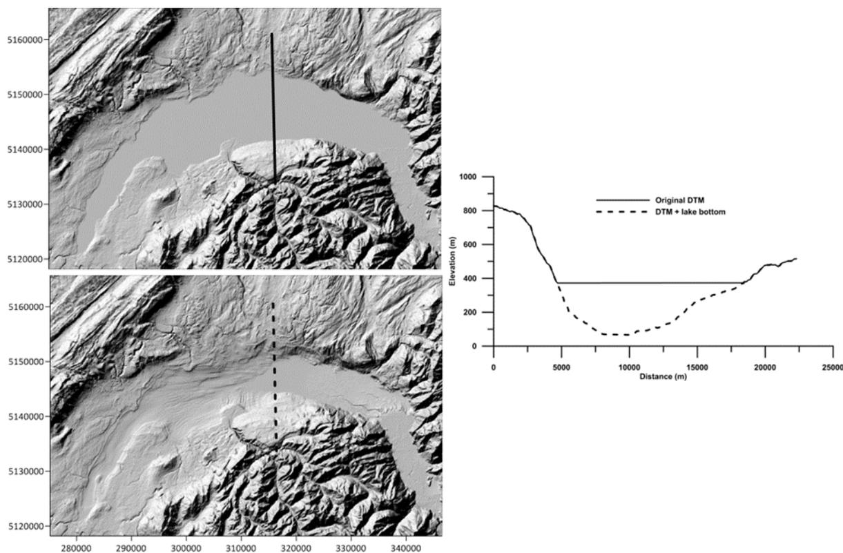
850 **Figure 14:** Examples of topography models used to calculate lake corrections (here, Lake Geneva, Switzerland). Top shaded relief represents the original DEM (MERIT), the bottom one the combination of DEM and lake bottom. The graph on the right shows two profile lines crossing both models (North is to the right).
