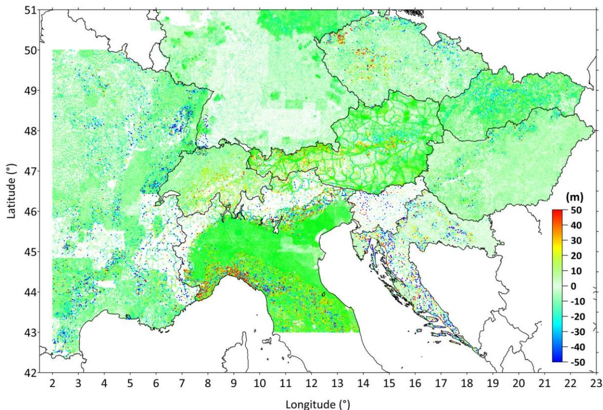
**Figure 6: Height differences (in meters) between MERIT DEM heights and heights of original surface gravity stations; MERIT DEM heights were considered for the “middle zone” of the mass calculation software TOPOSK (refer also to Sect. 4.1).**
