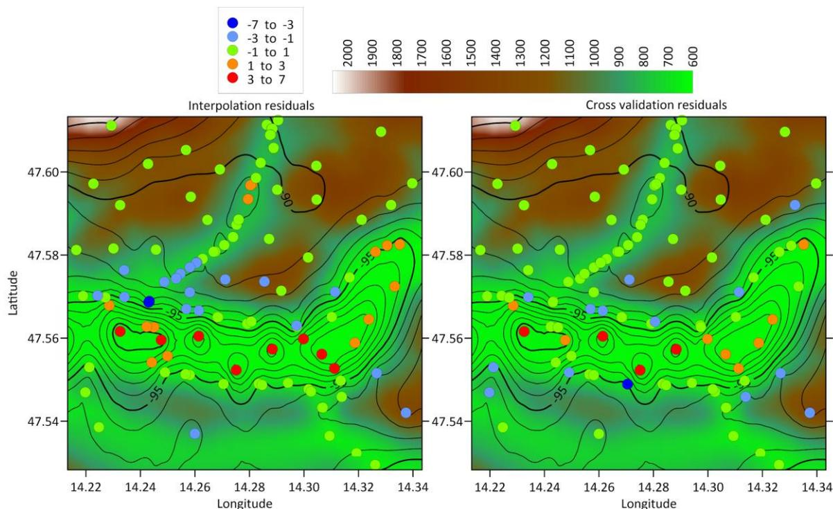
1295 **Figure 23: Interpolation and cross validation residuals of a subset within a small section of the Enns valley in Austria. Background: Topography, contour lines: CBA anomaly [mGal] interpolated using a high resolution grid (about 200 m spacing), coloured dots: residuals (left: interpolation, right: cross validation) at the scattered data points with respect to the AlpArray CBA grid (2000 m spacing). Residuals in [mGal], height in [m].**
