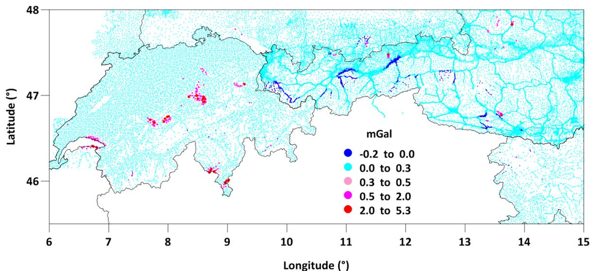
855 **Figure 15: Map of lake corrections (correction density is  $1670 \text{ kg m}^{-3}$ ). Small negative values occur in deep valleys with topography below the level of lakes (dark blue points).**
