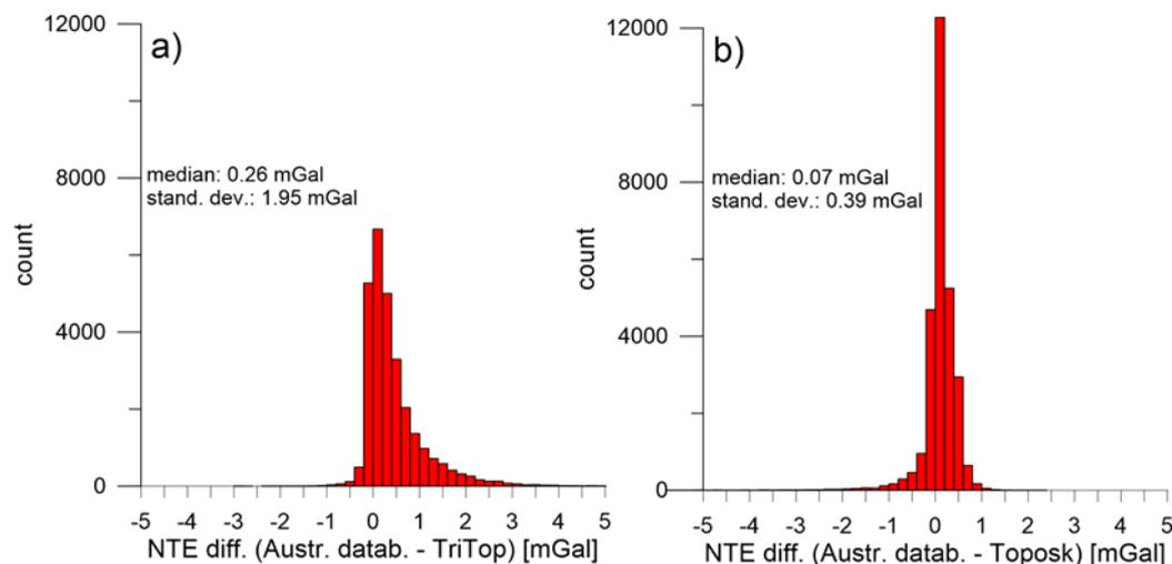
750 **Figure 8: Comparison of the differences between original mass corrections from the Austrian gravity database and NTE calculations by means of programs (a) TriTop and (b) Toposk.**
