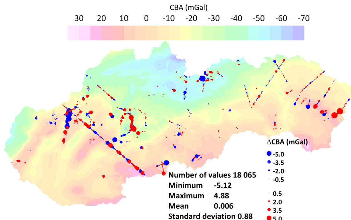
1205 **Figure 22: Differences between the CBA grid and independent gravity points (not used for the Slovakian part of the gravity grid compilation). It was calculated by SURFER's simple grid-residual procedure and showed that no gravity differences were greater than  $\pm 5$  mGal.**
