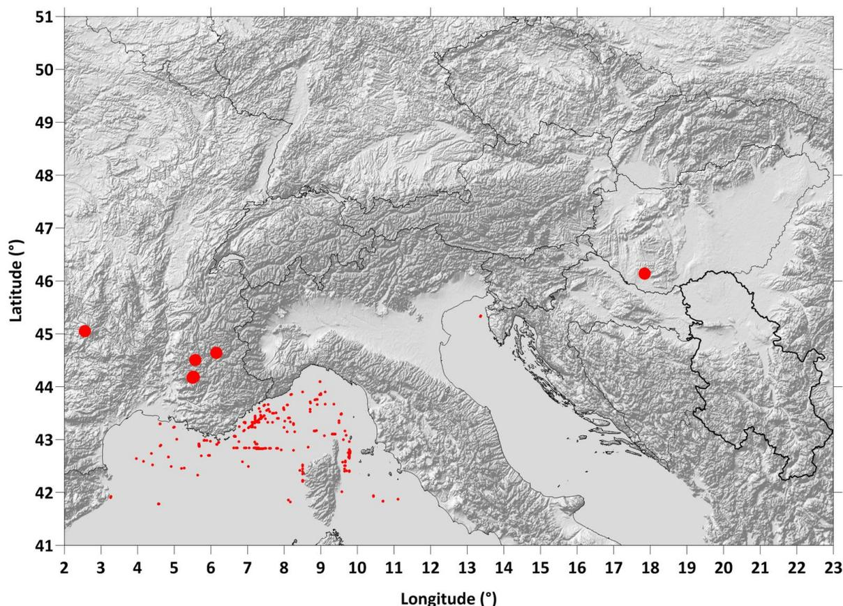
**Figure 26: Position of excluded points (733 points in total) based on interpolation residuals higher than  $\pm 10$  mGal. Almost all excluded points belong to marine data, very few points lie on land (enlarged points for clarity). The shaded relief in the background shows topography to distinguish land and offshore areas from each other.**
