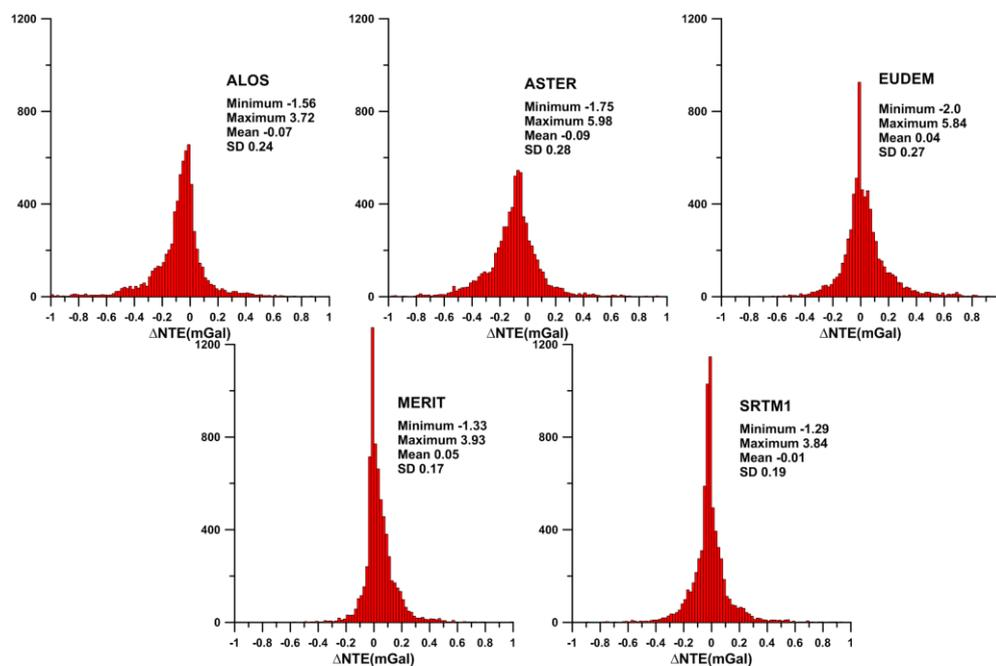
765 **Figure 9:** Near terrain effect (or mass correction, density  $2670 \text{ kg m}^{-3}$ ) differences calculated using various global models compared to the local Slovak terrain model DMR-3. The test was made on approx. 8000 points covering the whole territory of Slovakia.
