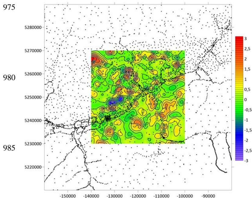
990 **Figure 19: Interpolation error estimate (gravity difference between gravity fields predicted by the EQS model and by 2D interpolation, contour interval 0.1 mGal, axis coordinates in [m] (Gauss-Krüger projection, M31).**
