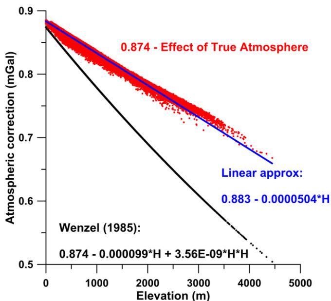
915 **Figure 17: Comparison of atmospheric correction at selected points covering the whole AlpArray area. The black dots represent the atmospheric correction calculated by a simple approximation according to Wenzel (1985). The red dots show the calculation using the effect of true atmosphere subtracted from the global constant value of 0.874 mGal (Mikuška et al., 2008) and the blue line is its linear approximation.**
