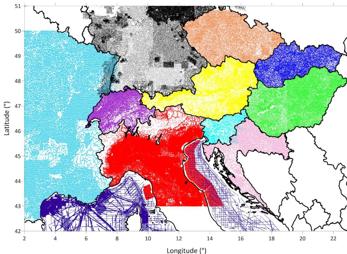
**Figure 1: The distribution of more than 1 million gravity stations in the area of investigation and compilation. Colours indicate the national databases used in the compilation. Starting on the left we designed: Light blue to France, black to Germany, orange to Czech Republic, dark blue to Slovak Republic, green to Hungary, pink to Croatia, red to Italy, dark blue to offshore areas, purple to Switzerland.**
