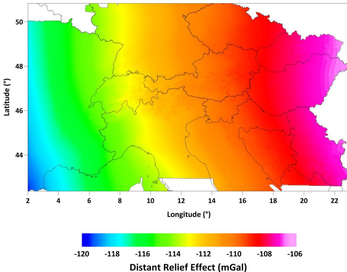
955 **Figure 18: The summary effect of topography and bathymetry (densities  $2670 \text{ kg m}^{-3}$  and  $-1640 \text{ kg m}^{-3}$ , respectively) from 166.7 km around the whole Earth.**
