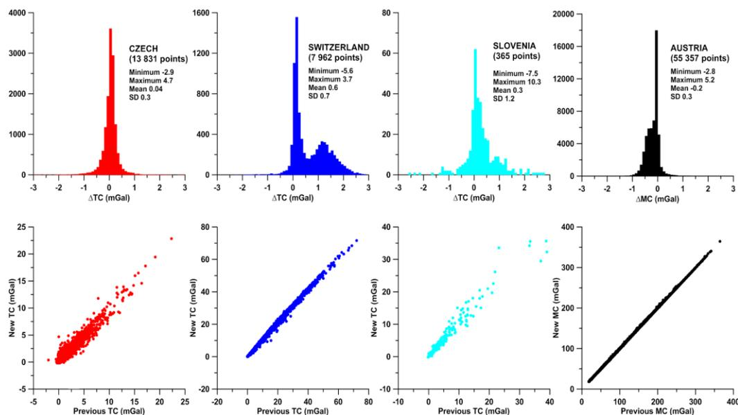
Figure 11: Comparison of original mass correction (or terrain corrections) values and values calculated using local DEMs. Note: There are different scales for each graph.
