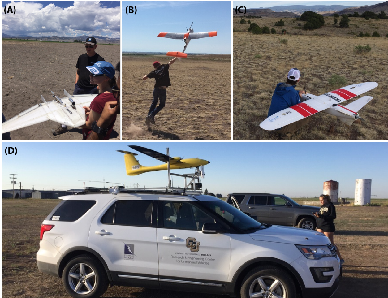
Figure 1: The aircraft used to collect the datasets described in this manuscript. Clockwise from top left: The CU DataHawk2, the BST S1, the CU Talon, and the CU TTWistor mounted on top of a tracker vehicle for launch prior to “follow me” operations.
