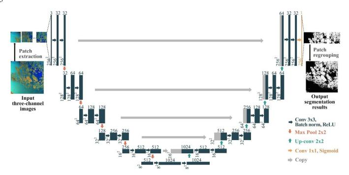
Figure 7. The overall architecture of the proposed sea ice segmentation model for the S1 EW data based on the U-Net deep learning algorithm.
