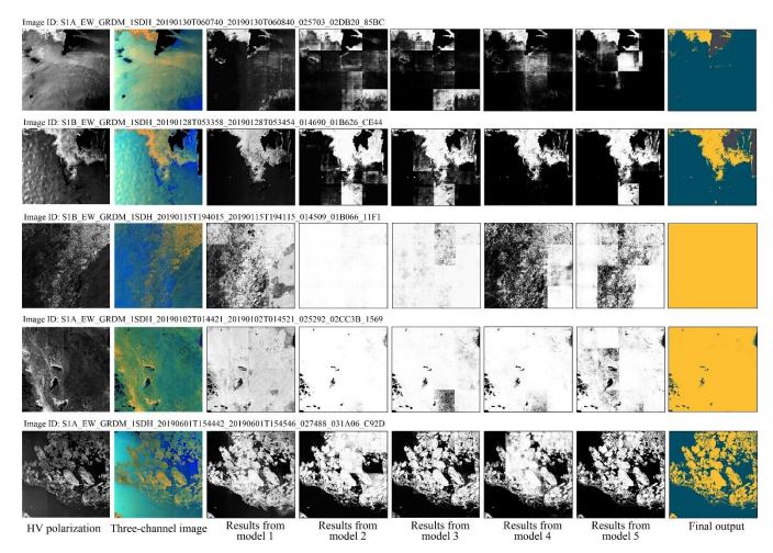
295 Figure 9. Five cases illustrating the combination of selected U-Net classifiers into the integrated stacking model. The first two columns are S1 images in HV polarization and the corresponding input RGB false-color composites. The following five columns are the outputs from the selected five classifiers with diverse specializations, and the last column is the final output of sea ice cover (yellow and cyan represent sea ice and open water, respectively).
