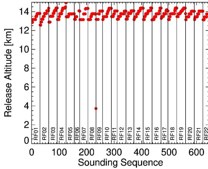
335 **Figure 5:** Time series of the release altitudes during OTREC. Sonde were typically launched above 12.1 km. Vertical lines separate the research flights, which are indicated near the bottom. The last sounding of RF08 was launched at low altitude due to operational reasons.
