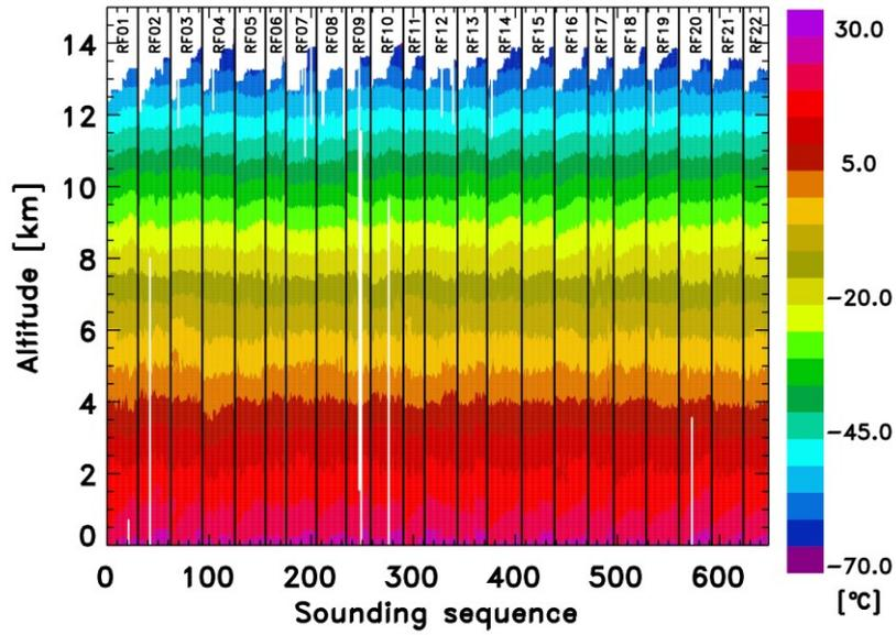
**Figure 9:** Color contours for all temperature measurements. Missing data are shown in white. All soundings are shown in the sequence in which they were released. Vertical lines separate the research flights, which are indicated in each group.
