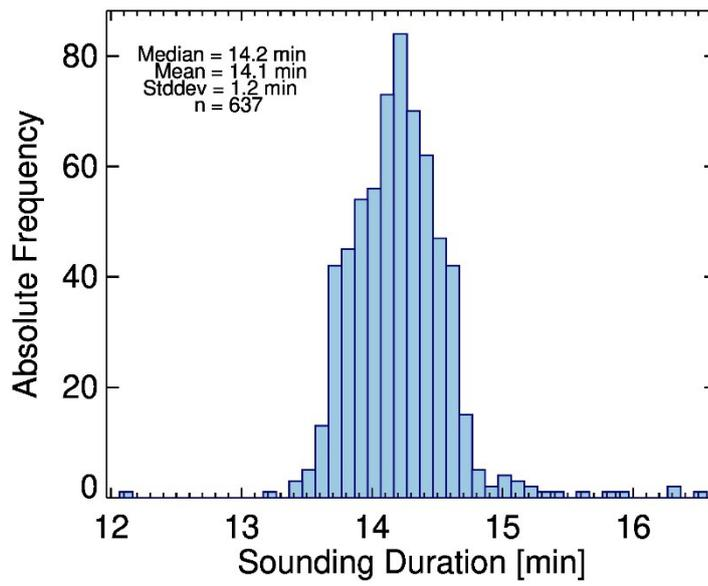
345 **Figure 8:** Measurement duration for all dropsonde with normal parachute behavior reaching the surface.
