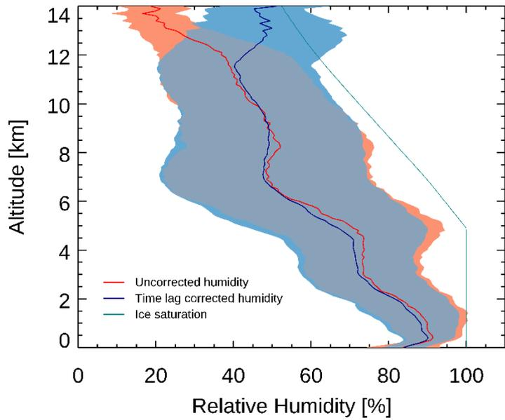
330 **Figure 4:** Mean relative humidity profile for all OTREC soundings. The average of the uncorrected relative humidity is shown in red, the average of the time lag corrected relative humidity is shown in blue. The standard deviation for each is shown as shaded areas. Saturation over ice is shown as solid green line.
