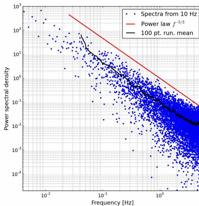
403 **Figure 15.** Example of turbulence spectra for the along wind component during a northerly storm with ~25 m/s mean
