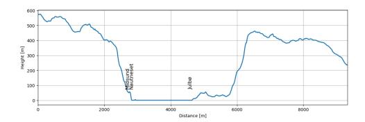
Figure 6 Terrain profiles along the sections indicated in Fig. 5, with the locations of the masts indicated. Terrain data are © Kartverket and licensed under Creative commons version 4.
