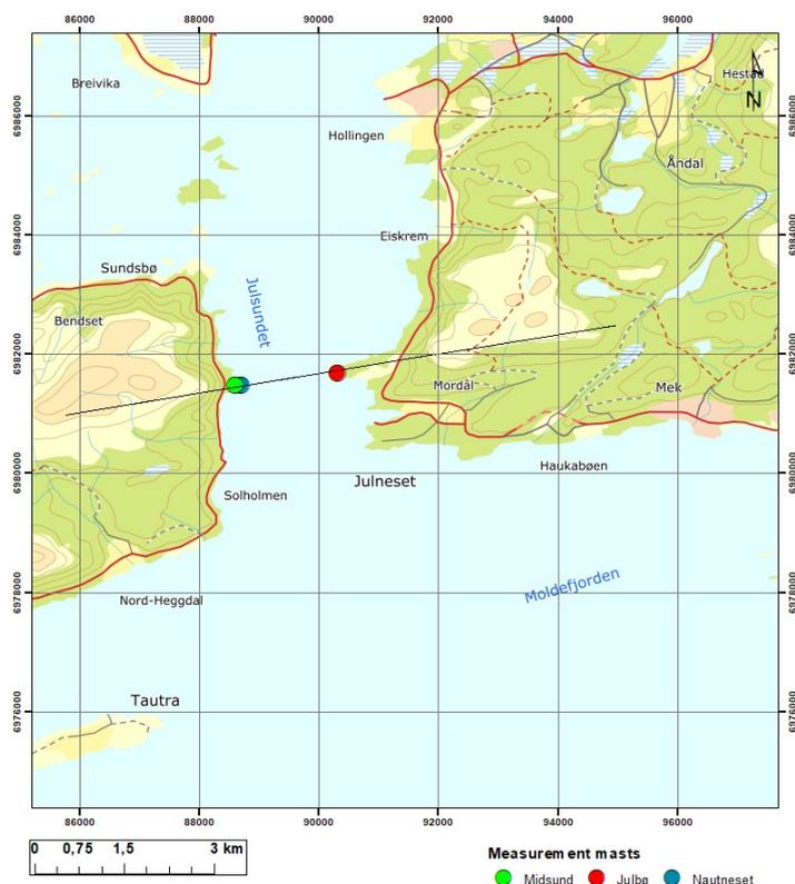
378 **Figure 5. Map of Julsundet with location of meteorological masts and the height profile shown in Fig. 6. Map layers**
