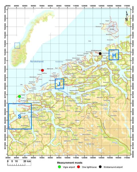
Figure 1. Overview of a part of the Møre and Romsdal region (approximate location shown in the inset) and the location of the three areas where the meteorological masts are located (S, J and H). The locations of three national weather stations with long-term data available, are indicated with coloured circles. Map layers are © Kartverket and licensed under Creative commons version 4.
