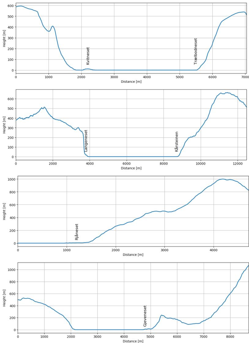
373 **Figure 3. Terrain profiles along the sections indicated in Fig. 2, with the locations of the masts indicated. Terrain data**
