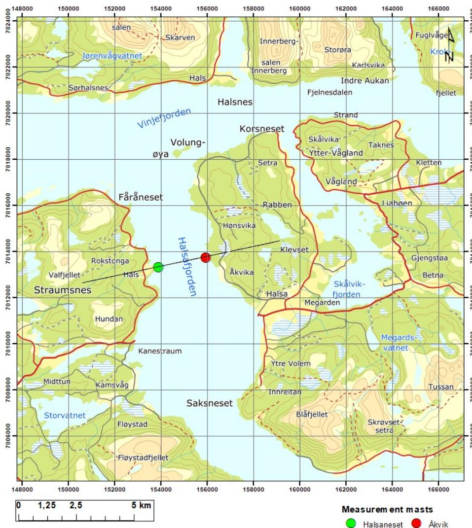
382 **Figure 7. Map of Halsafjorden with location of the meteorological masts, and the height profile shown in Fig. 8. Map**
