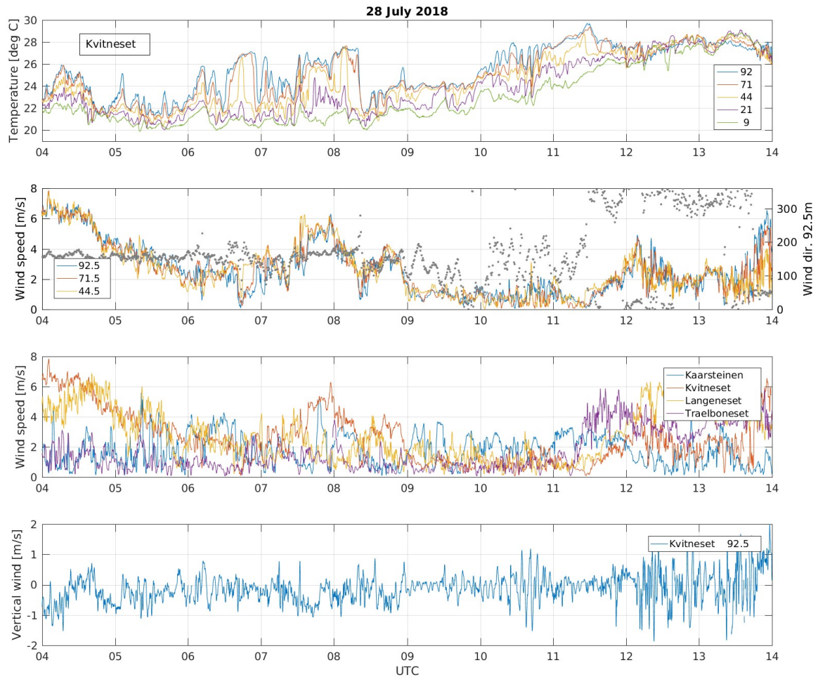
469 Figure 14. Time series of temperature, wind direction, horizontal and vertical wind speed at Kvitneset (panel 1, 2 and 470 4 from top) and horizontal wind speed from the top sensor of all four masts in Sulafjorden (panel 3). Sensor heights 471 at Kvitneset are given in the legends. The 10 Hz wind speed data are smoothed using a 30 s median filter.
