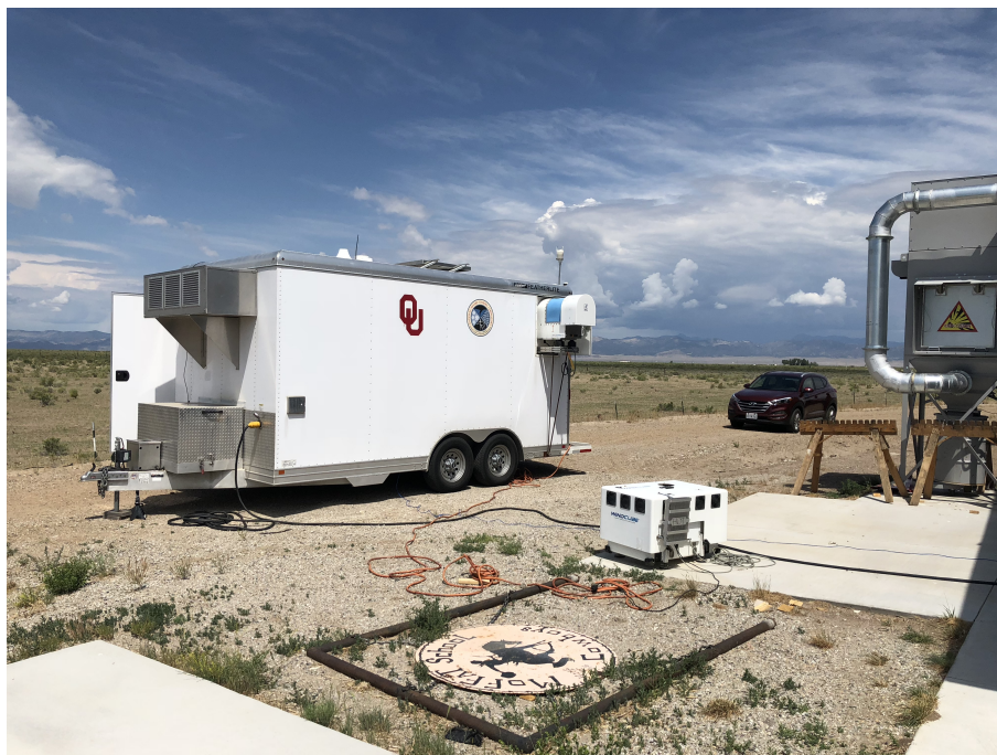
Figure 1. This photo shows the CLAMPS facility (white trailer) and the CU DPLR2 (foreground on the concrete pad) deployment location next to the Moffat school. Note, due to the proximity of the CLAMPS trailer to the building, the wind speed and wind direction from the meteorological station on the back of CLAMPS should be used cautiously.
