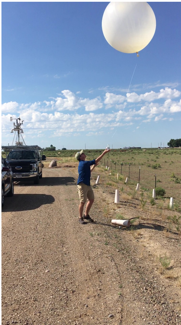
Figure 3. A radiosonde launch at Moffat School by Tyler Bell with the CLAMPS trailer. Photo credit Dr. Sean Waugh, NOAA/NSSL.
