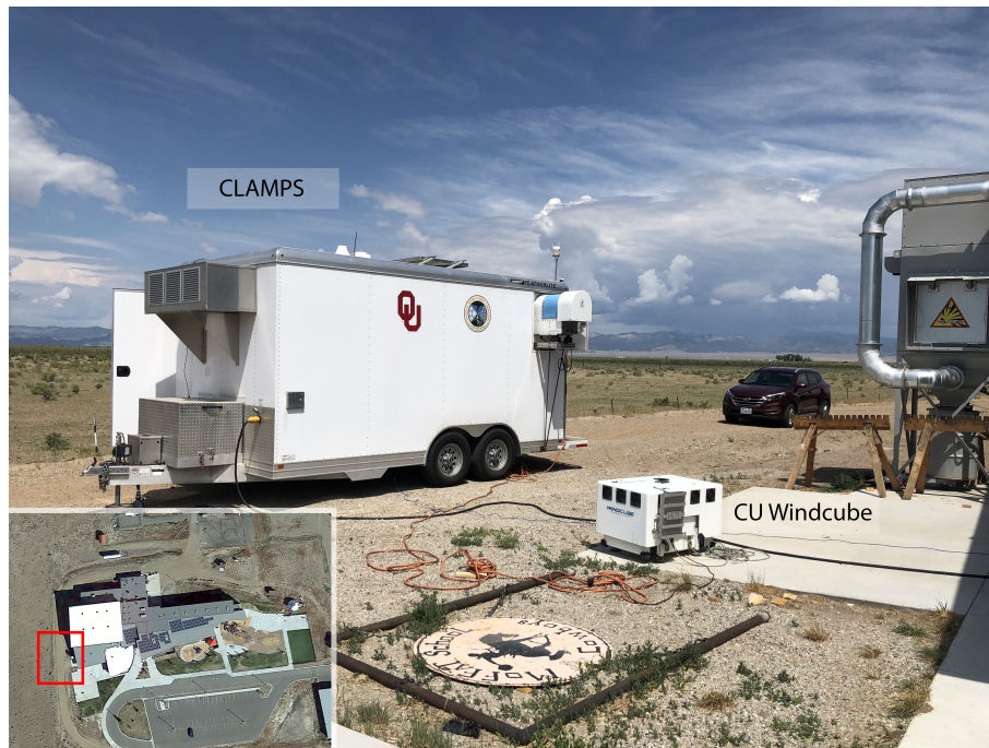
Figure 1. This photo shows the CLAMPS facility (white trailer) and the CU DPLR2 (foreground on the concrete pad) deployment location next to the Moffat Consolidated School. The red box on the satellite view shows where CLAMPS and DPLR2 were deployed in relation to the school building. Note, due to the proximity of the CLAMPS trailer to the building, the wind speed and wind direction from the meteorological station on the back of CLAMPS should be used cautiously. Satellite imagery ©Google Maps
