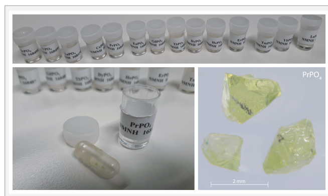
Figure 1. The reference REE orthophosphates from the National Museum of Natural History, example \text{PrPO}_4
