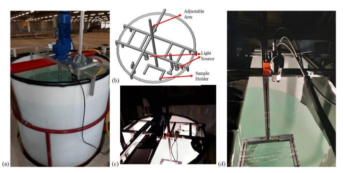
Figure 1. (a) Original set-up of the tank, (b) schematic of the aluminium frame, (c) experimental set-up of the tank inside covered with black cloth, and (d) foreoptic ends of the ASD and SEV spectroradiometers.
