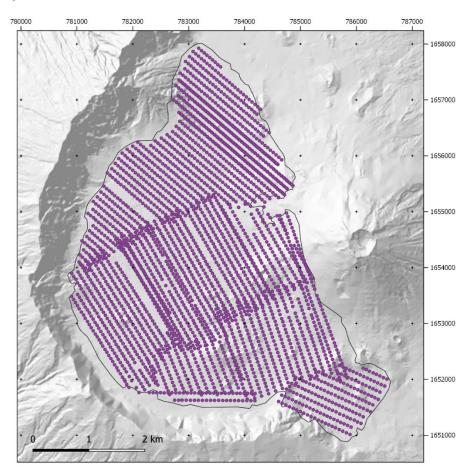
Figure 3 – Aerial survey of the Chã das Caldeiras with the geolocation of the photographs, Shaded relief derived from the DEMFI (2010) 5 m DEM.
