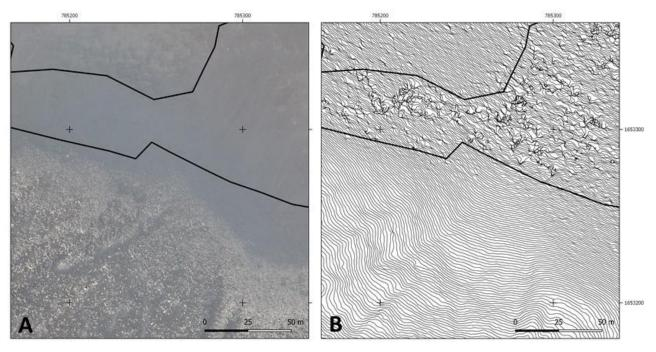
Figure 10 – Steep slope covered with ash in the Chã das Caldeiras with medium-quality results for the digital surface model. A. orthomosaic (10 cm resolution), and B. contour lines derived from the digital surface model (50 cm equidistance). The black line shows the boundary of the medium-quality area. The contours are very irregular in detail, but the overall slope at a coarse resolution is maintained. The area where the deposits are coarser provide a good DSM.
