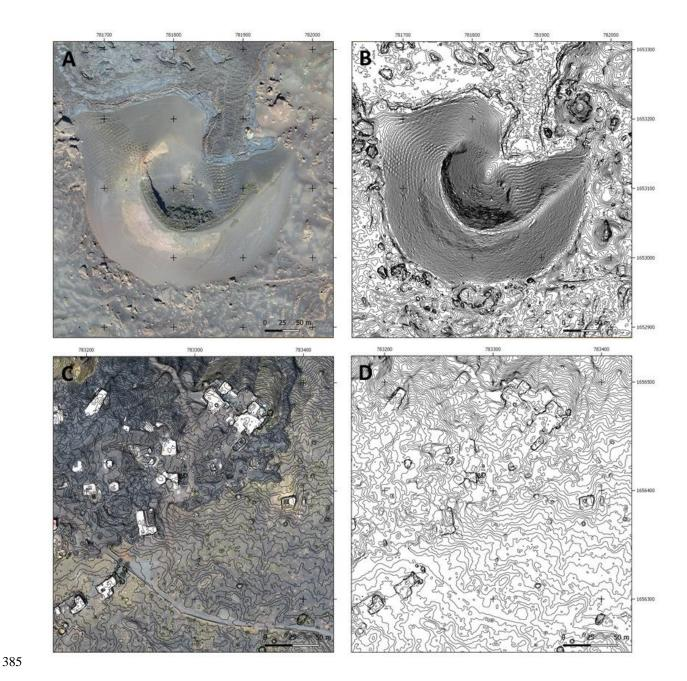
Figure 9 – Examples of surfaces in the Chã das Caldeiras with high-quality results for the digital surface model, with orthomosaic for visualization (10 cm resolution) and contour lines derived from the digital surface model (50 cm equidistance). Note the good quality of the elevation contours. A and B. Volcanic cone with cultivated areas inside the crater, C and D. Lava field with buildings and a road.
