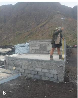
Figure 4 – Ground control point collection with RTK GNSS. A. Using markers, B. Using existing points.
