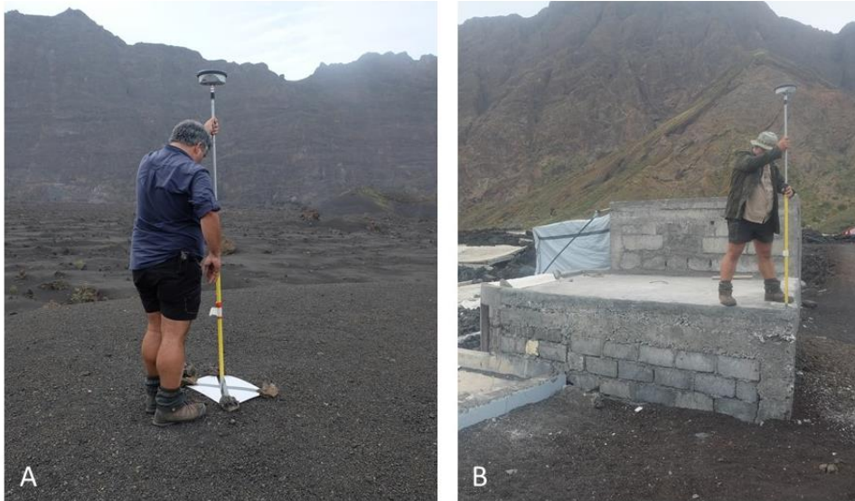
Figure 4—Ground control point collection with RTK GNSS. A. Using markers, B. Using existing points.
