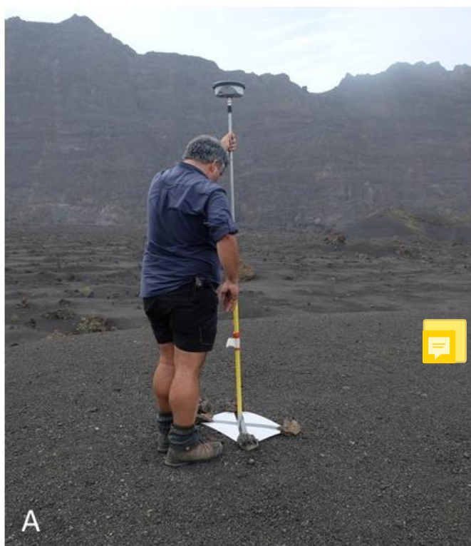
295 Figure 4 – Ground control point collection with RTK GNSS. A. Using markers, B. Using existing points.
