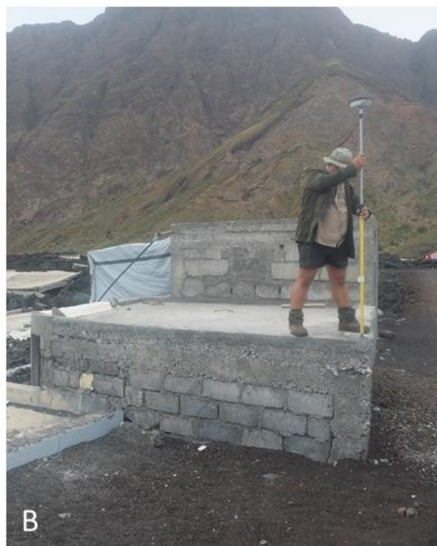
295 Figure 4 – Ground control point collection with RTK GNSS. A. Using markers, B. Using existing points.
