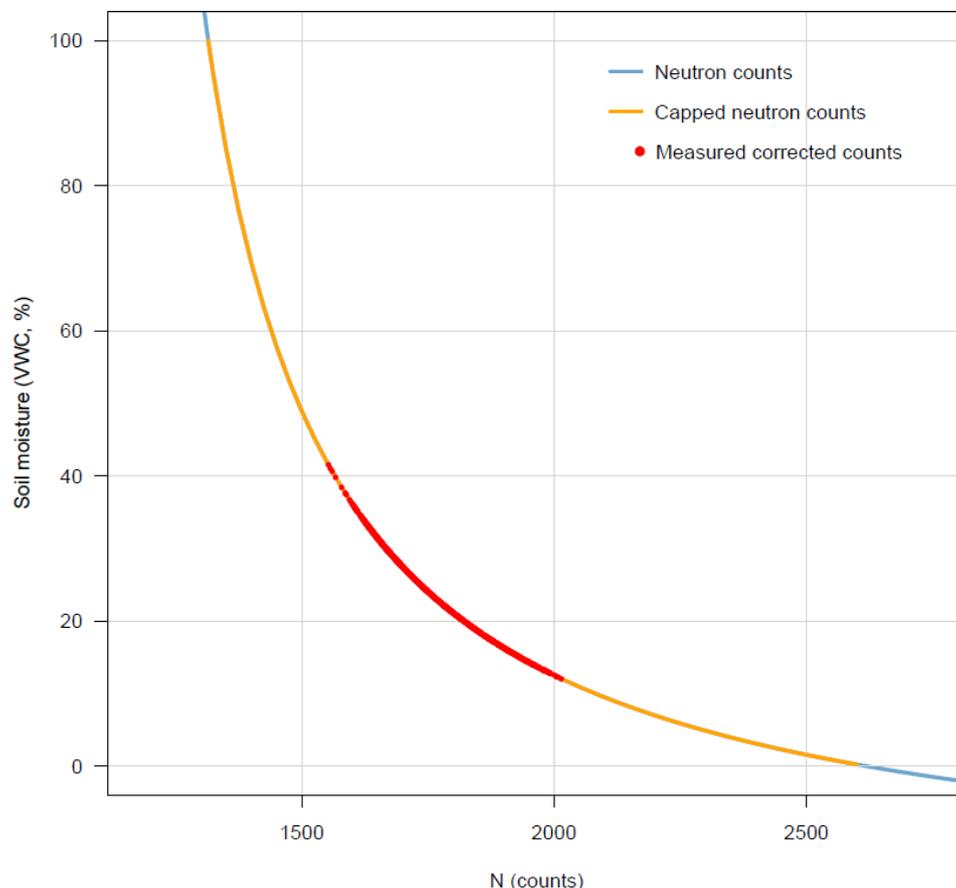
245 **Figure 4: CRNS VWC versus neutron counts for the Redhill site in South East England using the  $N_0$  technique is shown in blue.  $N_{\min}$  and  $N_{\max}$  for this site are 1314.75 and 2616.33 respectively as shown by the extent of the orange line. The range of measured corrected neutron counts at this site between 18 February 2016 and 01 September 2020 is shown in red.**
