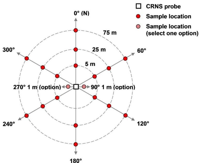
Figure 3: Plan view of soil sampling locations (not to scale).
