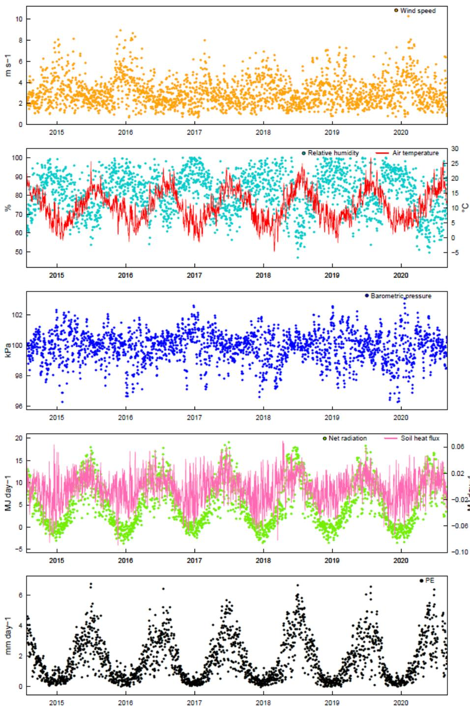
335 **Figure 8: COSMOS-UK observations required for the calculation of Potential Evaporation (PE) at the Rothamsted site in East Anglia.**
