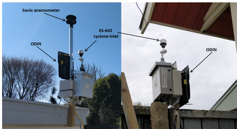
Figure 3. Examples of typical co-located ES-642 and ODIN installs. Note the instrument on the left is a Dust Met Mote with an additional sonic anemometer. An ODIN was co-located with every ES-642 instrument for intercomparison purposes.
