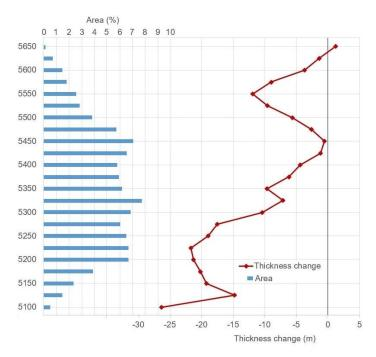
Figure 8: The mean thickness changes of Yala Glacier for 25 m elevation bands with hypsography, from 2000 to 2012. The reduced thickness change at an elevation of 5125 m is likely a result of the thinner ice thickness in the steeper part of the glacier in 2000. The increased thinning between 5525 and 5575 m a.s.l. might be caused by increased ablation at steep slopes and ice cliffs.
