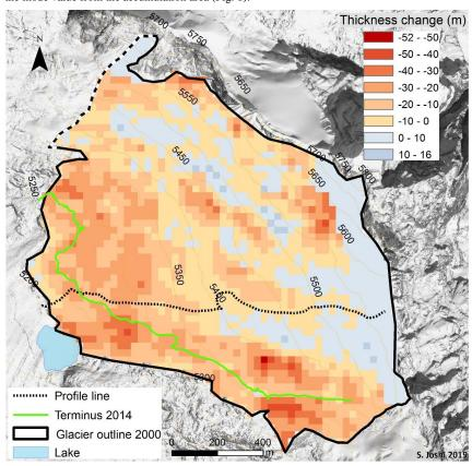
Figure 7: Thickness changes of Yala Glacier in metres after DEM differencing of GeoEye-1 (Jan 2012) and SRTM3 (Feb 2000) DEM and dGPS profile in 2012.
