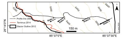
Figure 13: Glacier flow from 8 May 2012 to 5 May 2014 at the stakes 3, 4, 6 and 8, with annual rates between 4.6 and 7.8 m. The black arrows show the flow direction and the lengths indicate the annual speed of glacier surface flow, which is depicted 10 times longer than the real flow. The densely dashed line is the profile line from Sugiyama et al. 2013 (Figure modified from Sugiyama et al. 2013).
