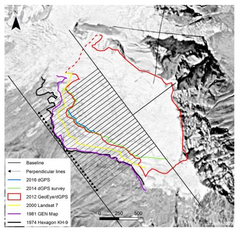
Figure 10: Frontal variations of Yala Glacier from 1974 to 2016. The general flow direction is indicated by a straight black line starting at the highest point of the glacier (north east corner). An arbitrary baseline is at the maximum extent of 1974 (black outline), and 26 parallel arrows in flow direction at 50 m intervals we used to calculate average front variations, but only the 9 bold lines were used for the analysis to exclude outliers. The background image is the Hexagon KH-9 from 1974.
