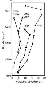
Figure 12: Altitudinal distribution of the surface flow speeds of Yala Glacier, surveyed in 1982 (solid diamonds, Ageta et al. 1984), 580 in 1996 (solid circles, Fujita et al. 1998), 2008 to 2009 (open circles, Sugiyama et al., 2013) and from 2012 to 2014 (solid tringle, this study) (modified Fujita et al. 1998).
