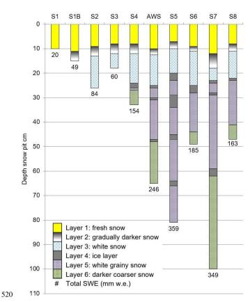
Figure 6: Snow profiles measured at the stakes on Yala Glacier on 23, 24 and 25 April 2017. At the site AWS, a temporary weather station was set up near stake S4. Distinct snow layers can be identified at all measurement sites. At the stakes S5, S6, S7, and S8 sawdust from 19 and 20 November 2016 was found at the bottom of the snow pit and glacier ice at all lower sites.
