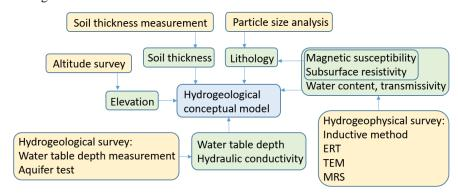
Figure 2. Fieldwork workflow for setting up a hydrogeological conceptual model at Maqu catchment.
