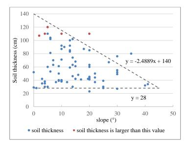
320 Figure 7. Soil thickness (m) vs. slope (°).
