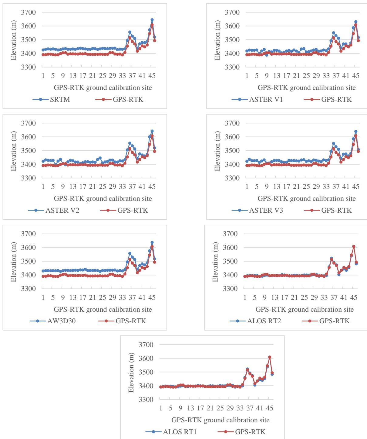
Figure 6. DEM elevations vs. GPS-RTK elevations.
