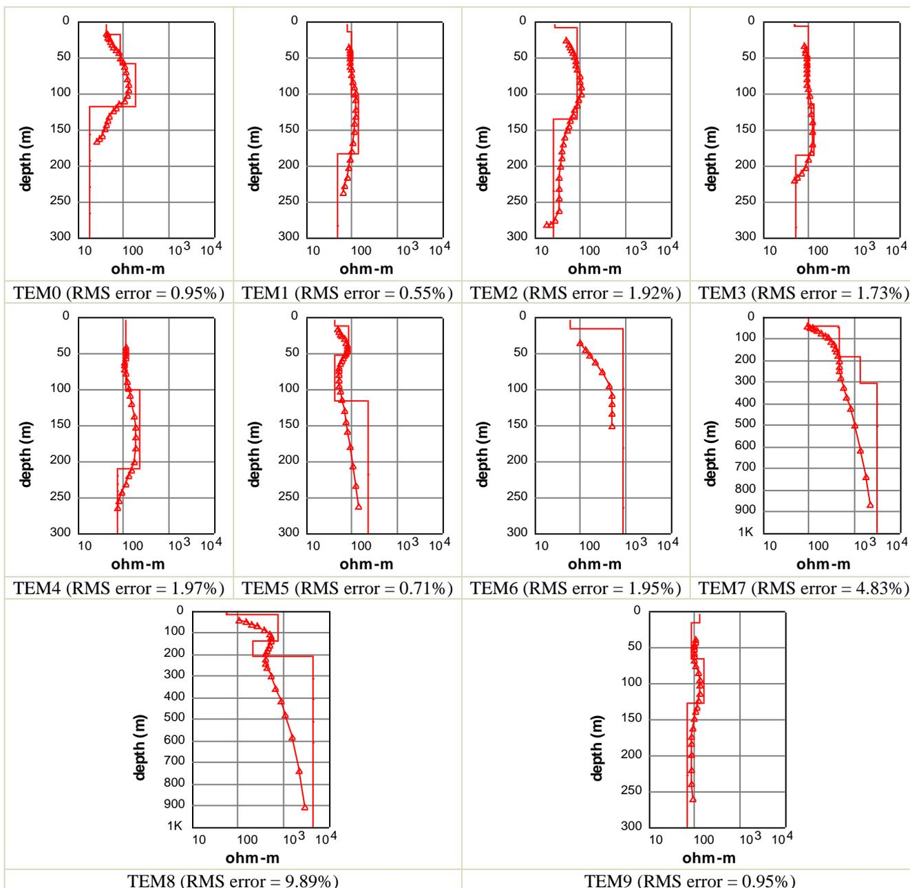
495 **Figure 13. Apparent resistivity and model of TEM.**
