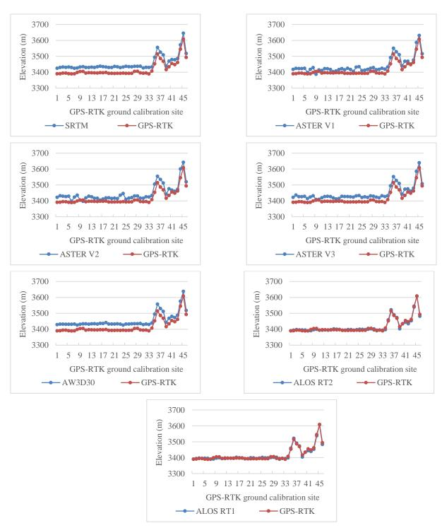
Figure 6. DEM elevations vs. GPS-RTK elevations.
