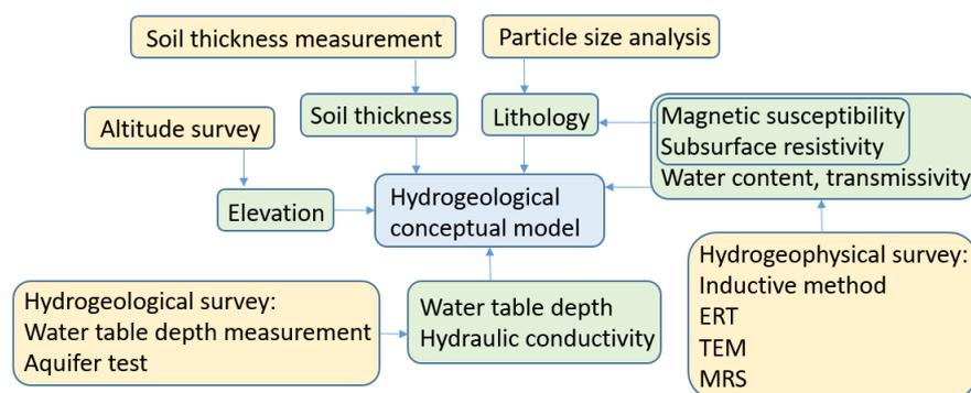
**Figure 2.** Fieldwork workflow for setting up a hydrogeological conceptual model at Maqu catchment.
