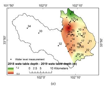
Figure 8. (a) and (b) are water table depths (m) of east Maqu catchment in 2018 and 2019, respectively; (c) and (d) are piezometric heads (m a.s.l) of eastern Maqu catchment in 2018 and 2019, respectively; (e) is the difference (m) of water table depth between 2018 and 2019. Numbers from 1 to 34 indicate boreholes listed in Table 6.
