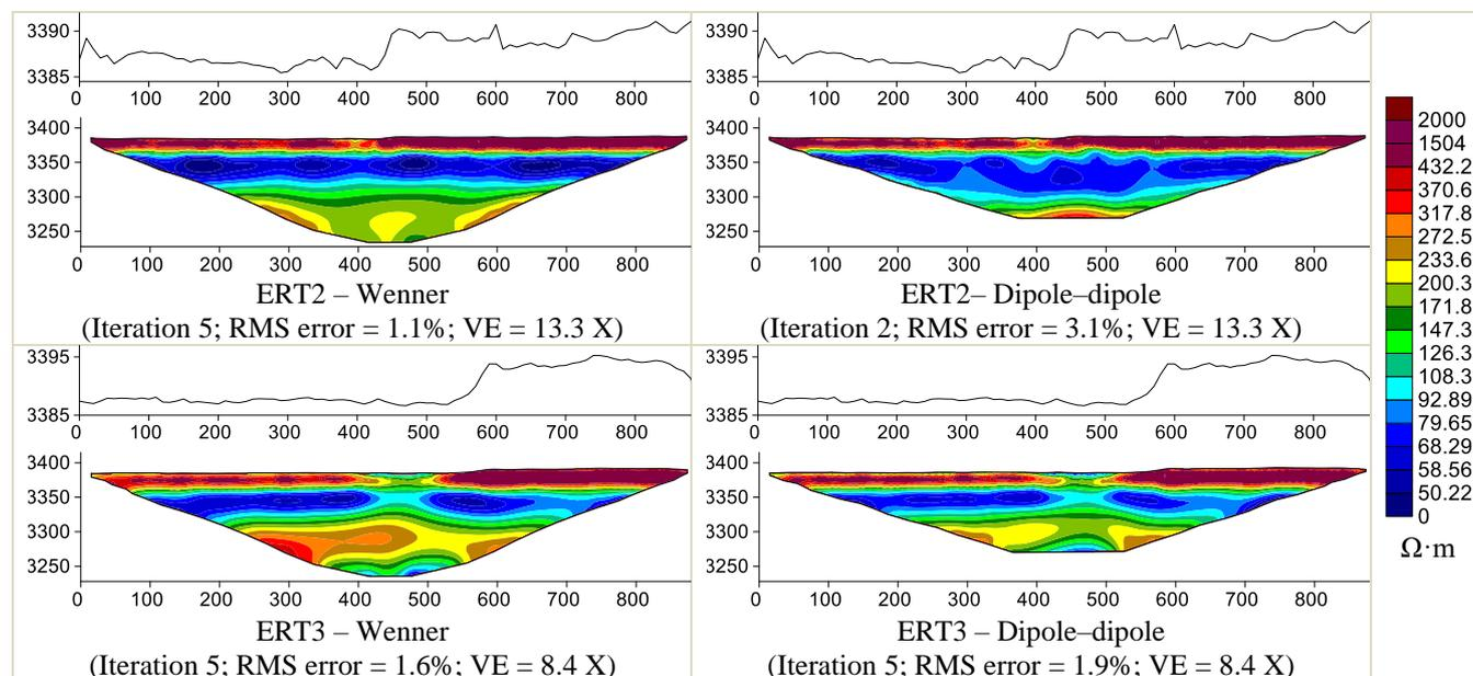
**Figure 11.** ERT2 and ERT3 measurements and corresponding ground surface elevation and vertical exaggeration (VE).
