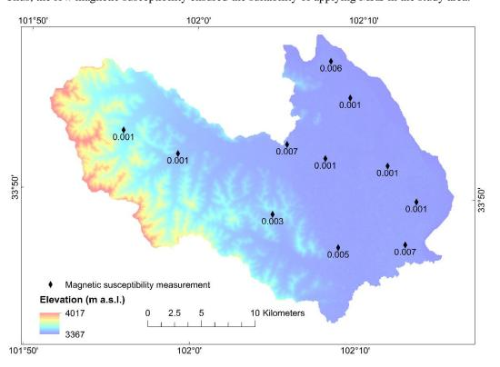
Figure 10. Magnetic susceptibility measurements (10<sup>-3</sup> SI Units) ensured the suitability of applying MRS in the study area.
