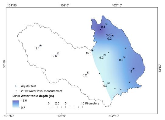
385 Figure 9. Hydraulic conductivity (m/d) obtained from aquifer tests, east of Maqu catchment.
