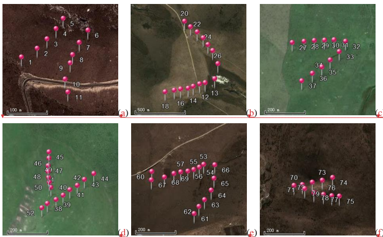
Figure 3. Locations of the hydrogeological surveys, ground surface elevation measurements, core lithology analysis, and soil thickness measurements. The numbers from 1 to 46 (due to limited space, several numbers are not shown in the figure) indicate the measurement sequence of GPS-RTK.
