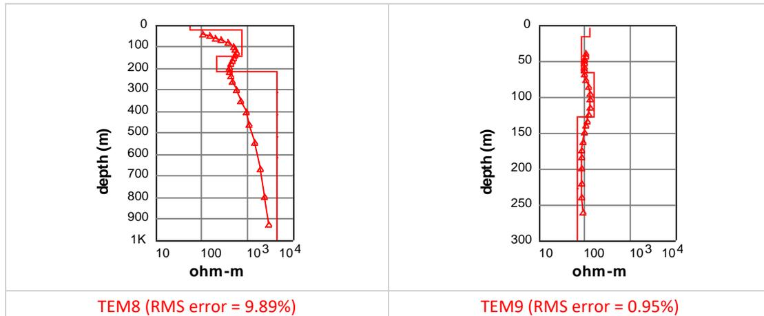
602 Figure 12. Apparent resistivity with depth. The red triangles connected by the red line
