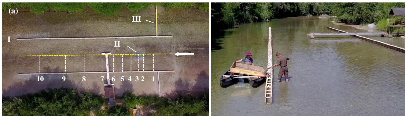
Figure 2. In-stream flume (a) aerial view of the flume (I is the wall of the flume, II is a model obstruction, II is a needle weir; the yellow dashed line is the longitudinal transect and white dashed lines are lateral profiles in a typical layout of experimental run), and (b) construction of the in-stream flume
