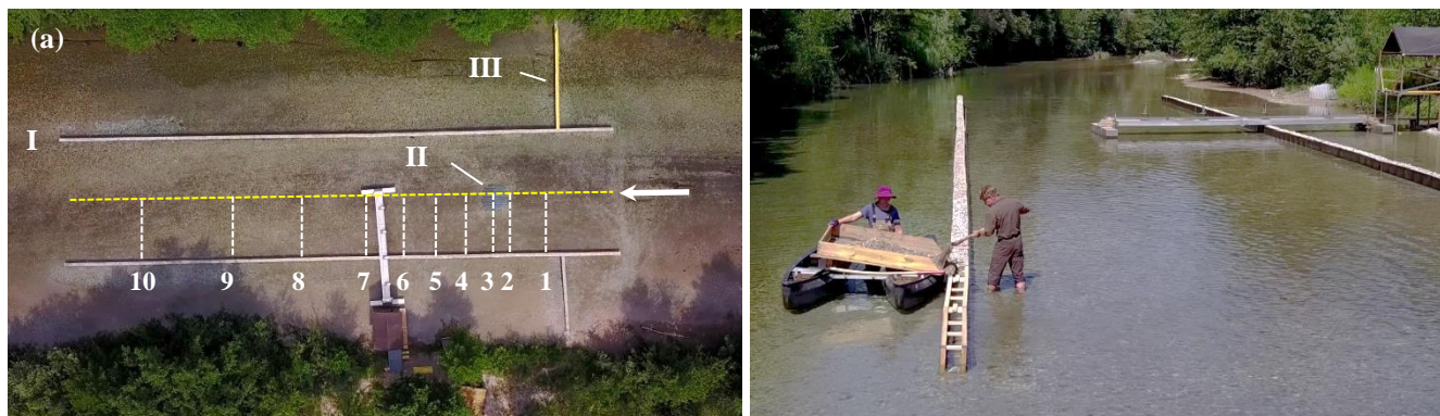
Figure 2. In-stream flume (a) aerial view of the flume (I is the wall of the flume, II is a model obstruction, III is a needle weir; the yellow dashed line is the longitudinal transect and white dashed lines are lateral profiles in a typical layout of experimental run), and (b) construction of the in-stream flume
