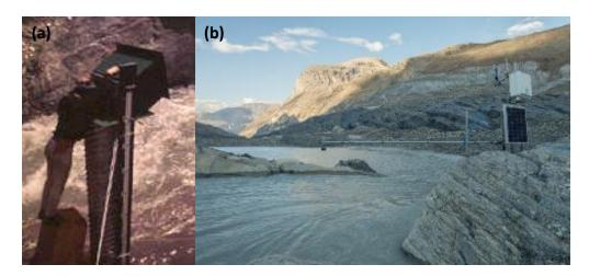
5 Figure 14: Gauge sites: (a) old IHD hydrometric gauge on Peyto Creek, August 1970 and (b) new hydrometric station at the Lake Munro outlet. Photographs by D. Scott Munro (a) and Angus Duncan (b).
