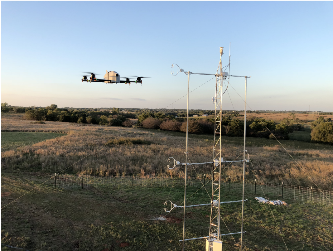
Figure 1. Photograph of the OU CopterSonde RPAS (Norman, OK, USA) in flight next to an experimental 10 m flux tower.
