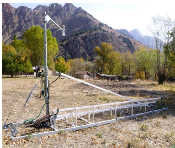
Figure 7: Snow Pack Analyzer (SPA) with the ultrasonic snow depth sensor (USH8) and the four flat ribbon sensors (three horizontal and one sloping sensor) at the station Maydantal (MTAL).
