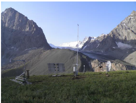
Figure 2: Station type one with meteorological sensors and a snow pack analyzing system (SPA, left front) at the station Golubin Glacier (GOLU)
