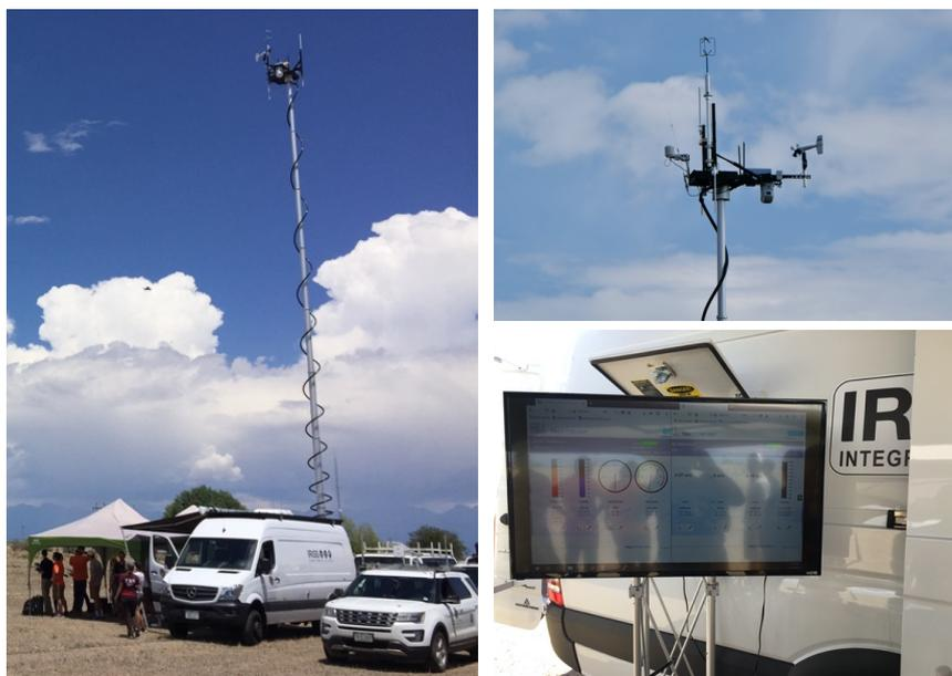
560 **Figure 1:** The CU MURC vehicle, with mast extended (left), as deployed during LAPSE-RATE. The right hand panels show the instrument cluster mounted on the top of the MURC mast (top) and the MURC real-time data display (bottom).
