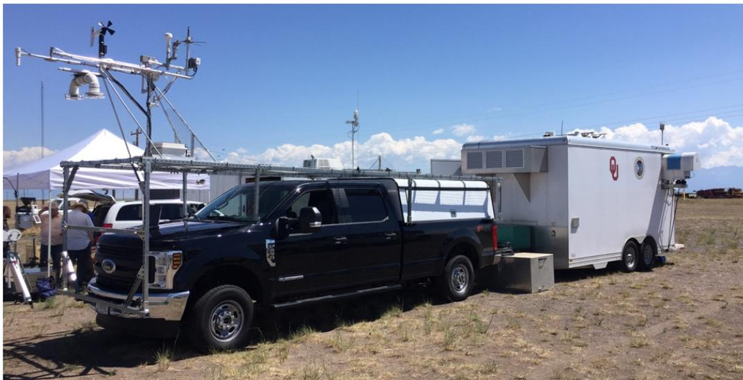
565 **Figure 2:** The NSSL MM as deployed during the LAPSE-RATE project. The trailer is the University of Oklahoma CLAMPS system (see Bell et al., 2020 in this special issue).
