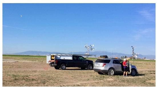
**Figure 4:** The NSSL MM and UNL CoMeT deployed side-by-side for an on-site intercomparison. The CU MURC was also located on site, but out of the photograph, and a CU TTwistor UAS (see de Boer et al., 2020c, in this special issue) flies in the background.
