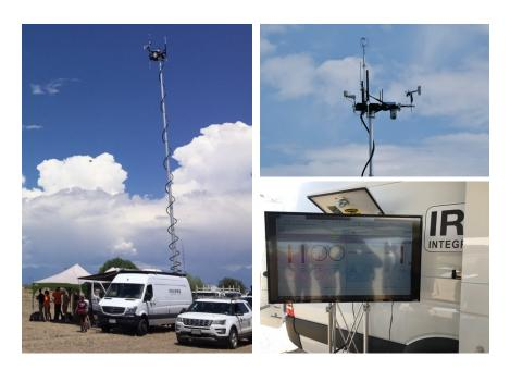
Figure 1: The CU MURC vehicle, with mast extended (left), as deployed during LAPSE-RATE. The right hand panels show the instrument cluster mounted on the top of the MURC mast (top) and the MURC real-time data display (bottom).
