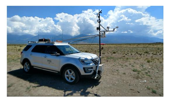
**Figure 3:** The UNL CoMeT vehicles, as deployed during LAPSE-RATE.
