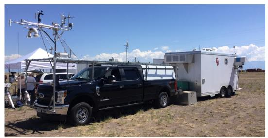
**Figure 2:** The NSSL MM as deployed during the LAPSE-RATE project. The trailer is the University of Oklahoma CLAMPS system (see Bell et al., 2020 in this special issue).
