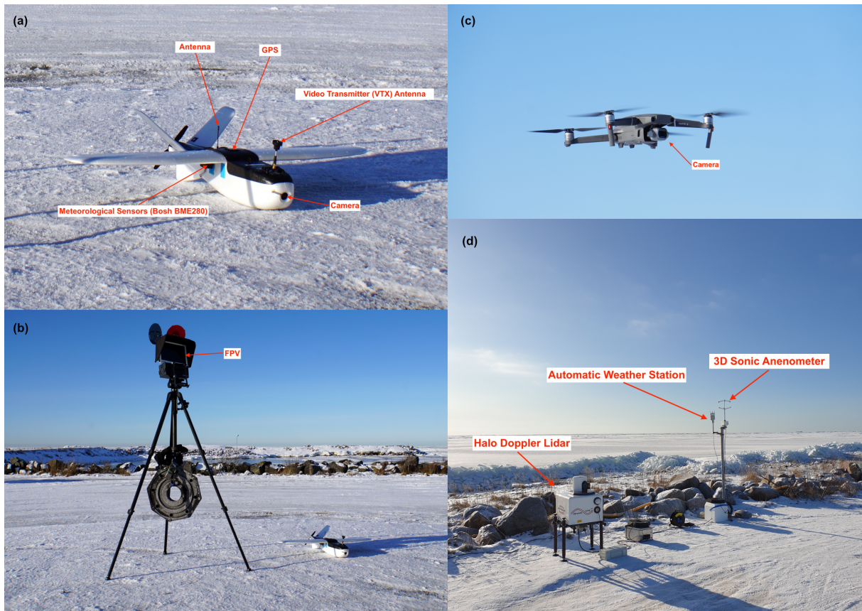
Figure 3. (a) UAV-UG1. (b) Telemetry screen for FPV real-time on-screen display of the UAV-UG1 performance. (c) DJI Mavic 2 Pro during flight. (d) Ground meteorological measurements.
