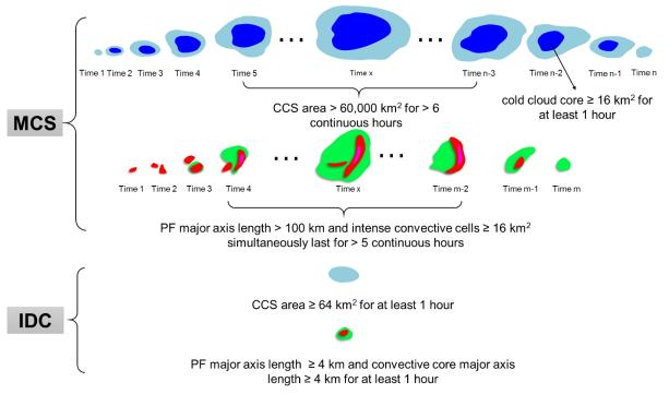
**Figure 4.** Definition of MCS and IDC based on the FLEXTRKR algorithm shown in Figure 3 and the specific threshold values used in the algorithm.
