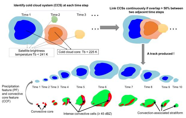
**Figure 3.** Schematic of the FLEXTRKR algorithm highlighting three key steps in the algorithm: (1) the identification of CCS (upper left), (2) linking of overlapping CCSs (upper right), and (3) the tracking of both PF and CCF (bottom).
