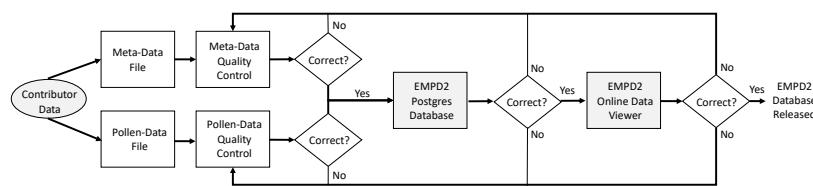
Figure 1. A flow diagram showing the data processing and quality control steps taken in constructing the EMPD2 database
