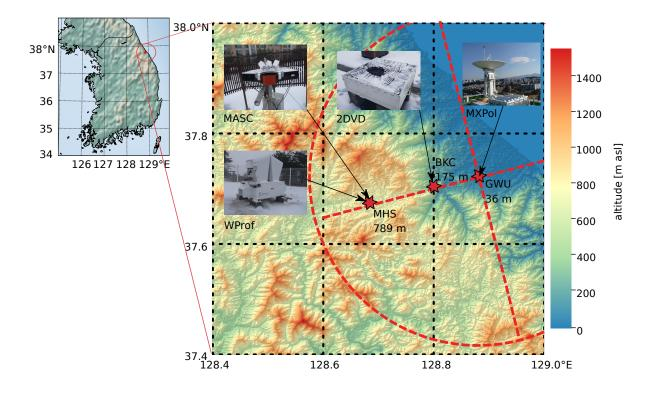
**Figure 1.** Location of the instruments used for this dataset. A digital elevation model shows the topography of the region and its location within South Korea. The red dotted lines and circle show the extent of the main RHIs (27.2 km) and PPI (28.4 km radius) respectively. Note that the MASC was located in BKC from 15 November 2017 to 20 February 2018 and in MHS afterwards.
