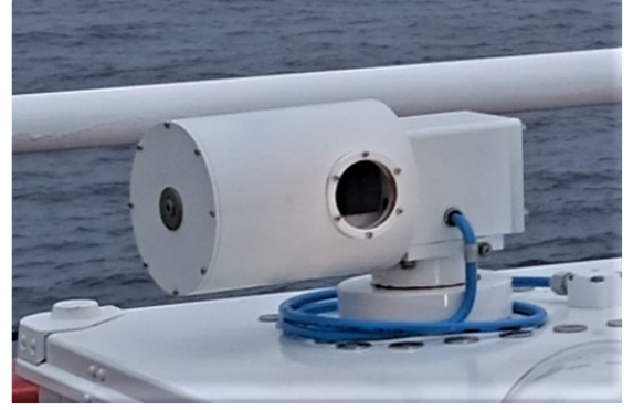
Figure 2. Photograph of the instrument container on board research vessel Sonne (left) and the solar tracker housing (right). The solar tracker housing (A on the left), the ambient sensors (B on the left), and the fisheye camera (C on the left) are mounted on top of the box. The solar tracker housing (right) consists of a cylinder which rotates around a horizontal axis in elevation direction. The cylinder is mounted on a cube which is able to rotate around a vertical axis in azimuth direction. Sunlight enters the tracker through a fused silica wedged window.
