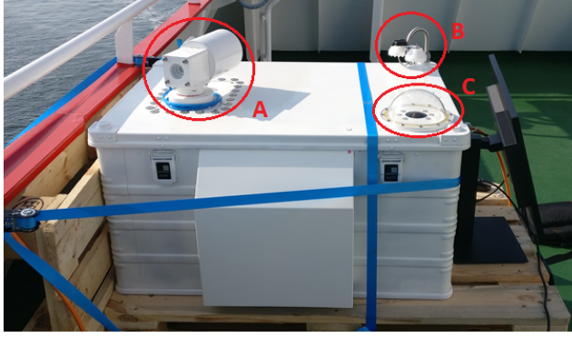
Figure 2. Photograph of the instrument container on board research vessel Sonne (left) and the solar tracker housing (right). The solar tracker housing (A on the left), the ambient sensors (B on the left), and the fisheye camera (C on the left) are mounted on top of the box. The solar tracker housing (right) consists of a cylinder which rotates around a horizontal axis in elevation direction. The cylinder is mounted on a cube which is able to rotate around a vertical axis in azimuth direction. Sunlight enters the tracker through a fused silica wedged window.
